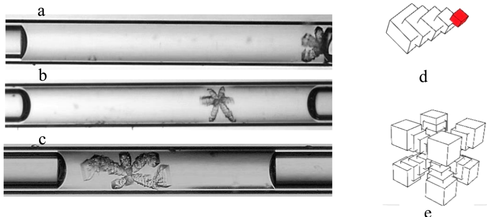
Figure 6. First appearance of crystals (5 s time-window) in (a) pure NaCl solutions, (b) the multibranch hopper formed in the NaCl solution with CTAB, and (c) the solution with Tween 80; when the hopper crystal grows rapidly and reaches the wall of the capillary, a change in the direction of the branches can be seen. (d,e) Illustration of hopper crystal with one branch and (e) star-like hopper crystal (multibranch) formed in bulk in the presence of CTAB and Tween 80.
