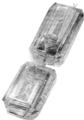
Figure 7.27. Two crystals resulting from one run still mounted on the silver seed holder and the baffle. [133]
