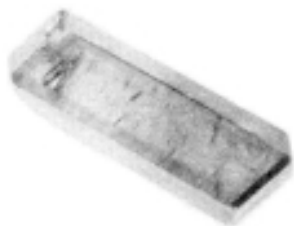
Figure 8.29. Sphalerite crystals grown under hydrothermal conditions. [99]
