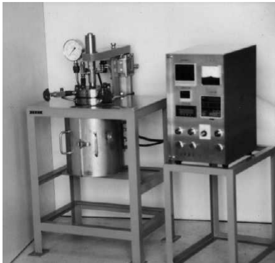
Figure 3.29. Commercially available autoclaves. (Courtesy of M/S Toshin Kogyo Co. Ltd., Japan.)
