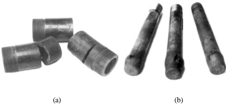
Figure 3.40. (a) Stellite Tuttle cold-cone sealed autoclaves and (b) stainless steel acid digestion bombs which ruptured at high pressure.
