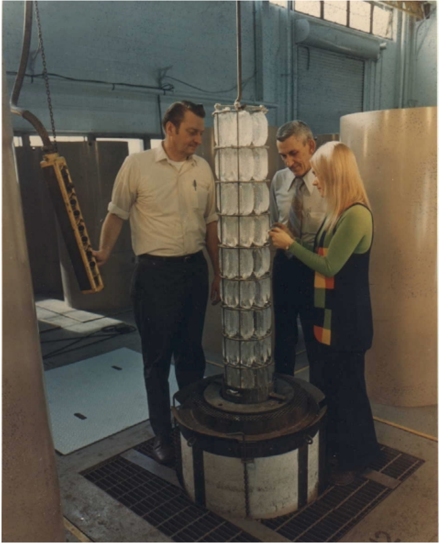
Figure 2.10. Quartz crystals obtained at AT&T Bell Labs. ( Photo courtesy of R. A. Laudise. )
