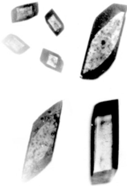
Figure 7.67. Photographs of \text{NaHZn}(\text{P}_2\text{O}_7) crystals (magnification \times 30 ). [301]
