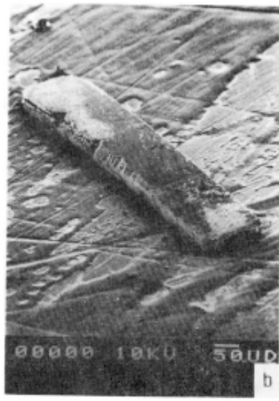
Figure 7.81. Photographs of \text{NH}_4\text{Zr}_2\text{V}_3\text{O}_{12} crystals obtained under hydrothermal conditions. [324]
