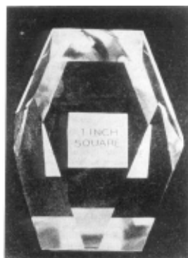
Figure 2.9. Quartz crystals obtained by Walker. [57]
