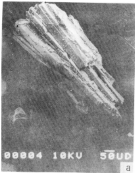
Figure 7.81. Photographs of \text{NH}_4\text{Zr}_2\text{V}_3\text{O}_{12} crystals obtained under hydrothermal conditions. [324]
