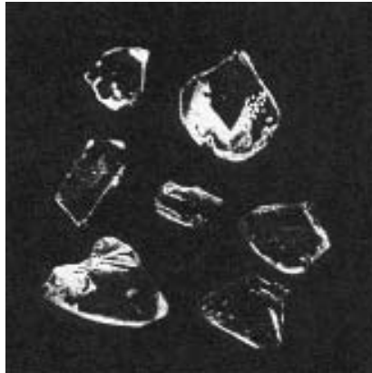
Figure 9.14. HfO 2 crystals. [73] (Courtesy of V. A. Kuznetsov.)
