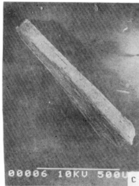
Figure 7.81. Photographs of \text{NH}_4\text{Zr}_2\text{V}_3\text{O}_{12} crystals obtained under hydrothermal conditions. [324]
