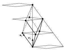
Figure 16.6. Primitive unit cell of the rhombohedral lattice 3R. The three fundamental translations  $\mathbf{a}_1$ ,  $\mathbf{a}_2$ ,  $\mathbf{a}_3$  are of equal length and make equal angles with  $\mathbf{e}_3$ . Hexagonal nets in four successive layers show how the rhombohedral cell may be constructed.
