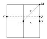
Figure 16.14. Brillouin zone of the reciprocal lattice of the strictly 2-D square lattice. The symmetry points mark out the basic domain; Z' and Z are equivalent points.
