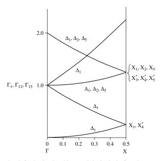
Figure 17.3. Energy bands for the simple cubic Bravais lattice in the free-electron approximation at  $\Delta$  on  $\Gamma$ X. The symmetry of the eigenfunctions at  $\Gamma$  and at X given in the diagram satisfy compatibility requirements (Koster *et al.* (1963)). Degeneracies are not marked, but may be easily calculated from the dimensions of the representations.
