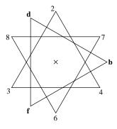
Figure 17.5. View looking down the [111] axis in Figure 17.4. The triangle containing 6, 7, 8 lies above the plane of the triangle containing the binary axes labeled **b**, **d**, and **f**, while that containing 2, 3, and 4 lies below this plane. Points marked 1 and 5 in Figure 17.4 lie on the axis through the center of this figure.
