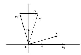
Figure 16.7. Action of the Seitz operator ( $R|\mathbf{v}$ ) on the vector  $\mathbf{r}$ . In this example, R is  $R(\pi/2 \ [0\ 0\ 1])$  and  $\mathbf{v} = \mathbf{a}_1/2$ . The dashed line shows  $\mathbf{r}' = R\mathbf{r} + \mathbf{v}$ .
