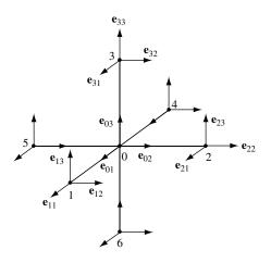
Figure 9.3. Basis vectors used to describe the atomic displacements in the  $ML_6$  molecule, showing the numbering system used for the seven atoms. (Labeling of the unit vectors at atoms 4, 5, and 6 is not shown explicitly to avoid overcrowding the figure.)
