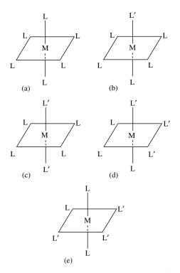
Figure 2.21. Configurations of an  $ML_6$  complex ion and of some  $ML_nL'_{6-n}$  complexes.
