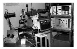
Fig. 12.5. A photograph of the double crystal X-ray diffractometer designed and developed at NPL
