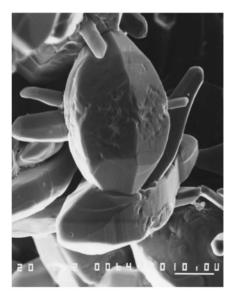
Fig. 11.9. SEM photograph of  $\beta$ -quartz crystal (Type 2C). 10 wt% NaCl solution, soaked at 700°C, and quenched at 650°C
