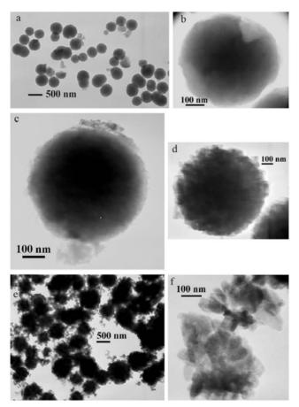
**Fig. 9.7.** TEM micrographs of (a) and (b) spherical hydrous titania precursor, (c) and (f) partially reacted spherical  $PbTiO_3$  powder, (d) and (e) fully reacted spherical  $PbTiO_3$  powder [20]
