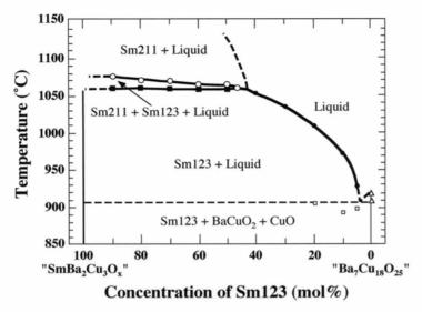
Fig. 14.27. Pseudo-binary phase diagram of the Sm123 system in air [37]
