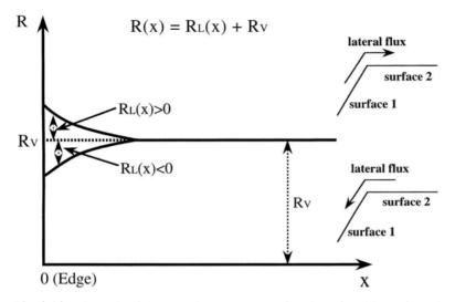
**Fig. 3.14.** Schematic of the growth rate R(x) as a function of position x from the boundary between two facets. R is the growth rate caused by lateral flux, and  $R_v$  is the growth rate caused by the direct flux.  $R_v$  equals the growth rate far from the boundary.
