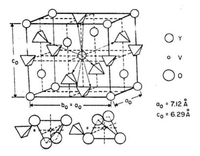
**Fig. 10.3.** Tetragonal unit cell of  $YVO_4$ .  $VO_4$  arrangements are represented by schematic tetrahedra: eight arrows indicate oxygen positions around the central Y of the YO<sub>8</sub> polyhedron [28]
