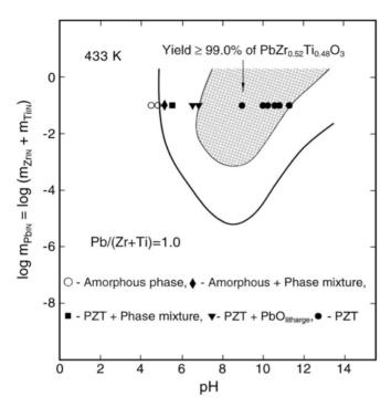
**Fig. 8.3.** Calculated yield diagram of  $PbZr_{0.52}Ti_{0.48}O_3$  at 433 K.  $PbAc_2$ ,  $TiO_2$ , and  $ZrO_2$  are used as starting materials for the calculations. Symbols denote various solid phases that were experimentally obtained using  $PbAc_2$  and coprecipitated the Zr-Ti hydrous oxide  $Zr_xTi_{1-x}O_2 \cdot nH_2O$
