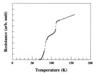
**Fig. 14.33.** Temperature dependence of the resistance of the sample annealed at 800°C in an oxygen atmosphere (Reprinted from [34(a)], with permission of Elsevier Science)
