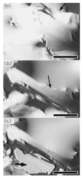
**Fig. 14.31.** Photographs of the plate crystals that appeared as the temperature decreased. The scale bar indicates 100  $\mu$ m. (a) The first crystals grown on the surface of a liquid (marked by an arrow) at 865°C. (b) The first crystals dissolved at 860°C. The solid-liquid boundary is marked by an arrow. (c) The second crystals (marked by an arrow) grew from the liquid at 845°C. (Reprinted from [34(a)], with permission of Elsevier Science)
