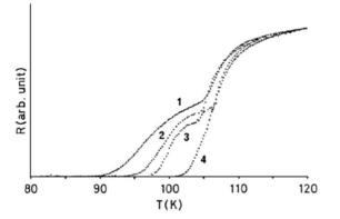
**Fig. 14.2.** Sintering time dependence of the *R*-*T* curves for the specimens that were sintered at 840°C for various periods of time. (1) 1 h, (2) 30 h, (3) 48 h, (4) 100 h. (From reference 2 by permission of *Jpn. J. Appl. Phys.*)
