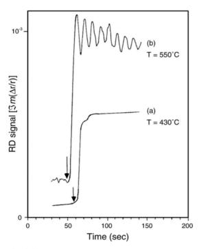
**Fig. 3.21.** RDS response of a (001) GaAs surface when TEG is supplied to an  $AsH_{3}$ -stabilized surface at (a) 430°C and (b) 550°C. The arrows indicate the event when TEG was injected into the growth chamber [41].
