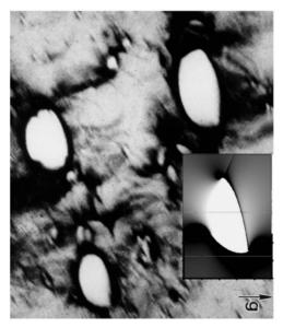
**Fig. 6.15.** 1126 grazing-reflection topograph of micropipes. Inset is the simulated contrast of a 4*c* screw dislocation with surface relaxation effect considered [97]
