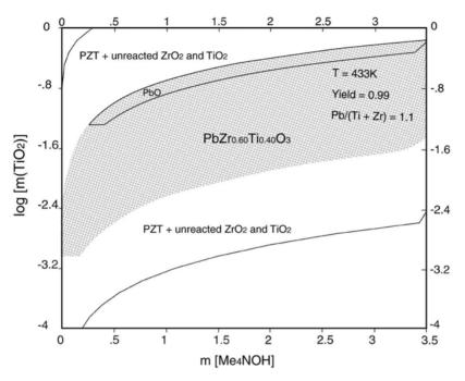
**Fig. 8.9.** Calculated yield diagram of  $PbZr_{0.6}Ti_{0.4}O_3$  at 433 K.  $PbAc_2$ ,  $TiO_2$ , and  $ZrO_2$  are used as starting materials for the calculations
