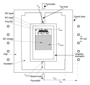
Fig. 6.6. Schematic of the SiC growth system
