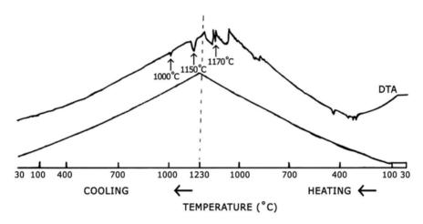
Fig. 12.9. A typical DTA curve recorded for lithium niobate powder
