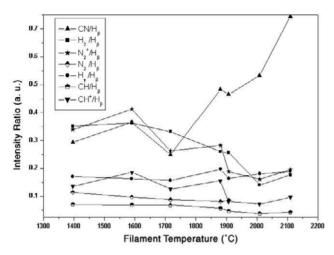
Fig. 4.18. Effect of filament temperature on the relative emission intensities [182]
