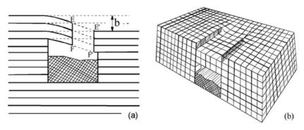
**Fig. 6.22.** Schematic diagram illustrating the creation of a pair of opposite-sign screw dislocations during the process of inclusion overgrowth. (a) Sectional view through the inclusion parallel to the dislocation line. (b) Perspective view from above [112]
