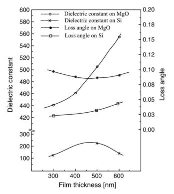
**Fig. 5.8.** Relative dielectric constant and loss angle measured from PNZT thin films on silicon and MgO substrates as a function of the film thickness (reprinted from Ref. 66 with permission from AIP)
