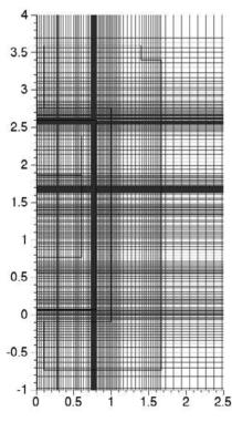
**Fig. 7.5.** Computational grids for finite volume method [13]. Grids are highly clustered in the regions of large temperature gradients.
