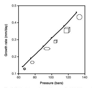
Fig. 10.14. Morphology variation with pressure for  $Nd:GdVO_4$  crystals
