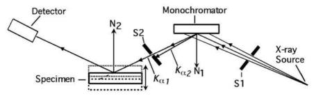
Fig. 12.6. A schematic diagram of the double crystal X-ray diffractometer developed at NPL
