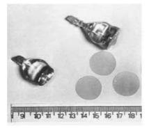
**Fig. 12.10.** LiNbO<sub>3</sub> crystals grown along the [00.1] direction. A few polished wafers cut perpendicular to the growth direction are also shown.
