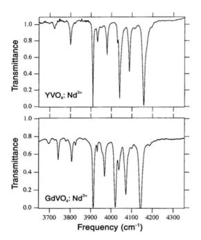
Fig. 10.21. Transmittance spectra for Nd- doped  $YVO_4$  and  $GdVO_4$  showing  ${}^4I_{9/2} \rightarrow {}^4I_{13/2}$  transitions [48]
