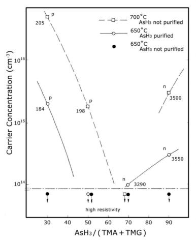
**Fig. 3.16.** Electrical properties of AlGaAs ( $X_{Al} = 0.2$ ) obtained from Hall measurements at RT: (Y) AsH<sub>3</sub> was purified ( $Tg = 650^{\circ}$ C), ( $\lambda$ ) AsH<sub>3</sub> was not purified ( $Tg = 650^{\circ}$ C), ( $\blacklozenge$ ) AsH<sub>3</sub> was not purified ( $Tg = 700^{\circ}$ C). The same AsH<sub>3</sub> cylinder and TMA (#1) were used throughout [22].
