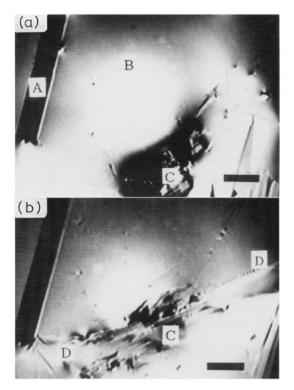
**Fig. 14.35.** Optical micrographs of the surface of the sample. Scale bars indicate 100  $\mu$ m. (a) After the temperature of the sample was kept at 870°C for 24 h. A: the needle crystal of (Sr,Ca)CuO<sub>2</sub>; B: surface of the liquid; C: crystals of the low *T<sub>c</sub>* phase. (b) 18 h after (a). D: newly grown plate crystals. (Reprinted from [34(b)], with permission of Elsevier Science)
