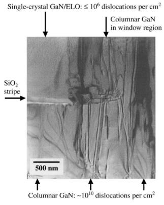
Fig. 3.32. Vertical-cross-section TEM image (g = (0001)) [68]
