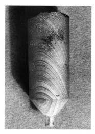
Fig. 15.5. ZnSe crystal grown by high pressure Bridgman method (from Reference 41)
