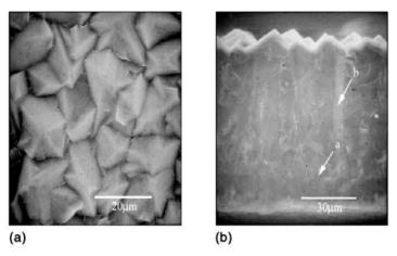
**Fig. 4.7.** SEM photographs of diamond film with the two-step growth method. (a) (110)-orientation diamond film and (b) the cross section of diamond film [130]
