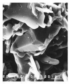
Fig. 11.7. SEM photograph of  $\beta$ -quartz crystal (Type 2N) without prism faces. 10 wt% NaCl solution, soaked at 750°C and quenched at 700°C. A black arrow indicates co-existing Type 1 crystal
