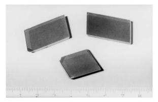
Fig. 15.13. (100) ZnSe substrates grown by solid-state recrystallization (from Reference 114)
