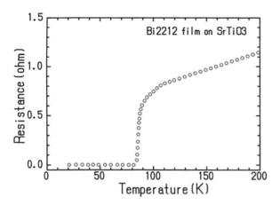
Fig. 14.19. Temperature vs resistance curve of the film grown for 20 hours. (From reference 28 by permission of the *Jpn. J. Appl. Phys.*)
