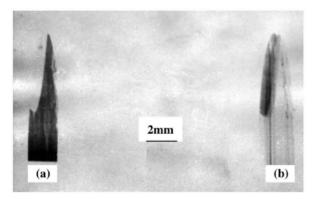
**Fig. 12.22.** Typical high resolution X-ray traverse topographs of the (001) BGO specimen of Figs. 12.17 to 12.21 recorded with (004) diffracting planes in symmetrical Bragg geometry. (a) and (b) were recorded after orienting the specimen on peak #1 and #2, respectively, of Fig. 12.21.
