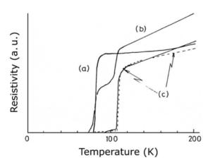
**Fig. 14.15.** Annealing temperature dependence of the *R*-*T* curves for the series A crystals (a) before and (b, c) after annealing at (b) 841°C and (c) 852°C. (From reference 4 by permission of *Jpn. J. Appl. Phys.*)
