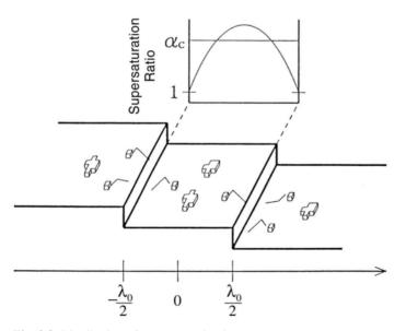
Fig. 3.8. Distribution of supersaturation between two steps
