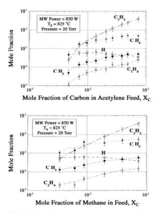
**Fig. 4.10.** Mole fractions measured at the substrate in a microwave plasma reactor as a function of carbon mole fraction in the feed gas  $X_c$ . (a), the carbon is introduced as acetylene, (b) the carbon is introduced as methane [147].
