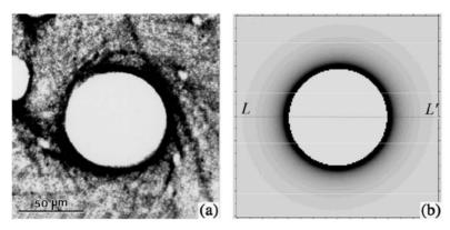
**Fig. 6.11.** (a) Back-reflection SWBXT image of an 8*c* micropipe taken from a (0001) surface of a 6H-SiC crystal. Sample-to-film distance 20 cm; (b) Simulation of a screw dislocation with Burgers vector  $|\mathbf{b}| = 8c$  [98]
