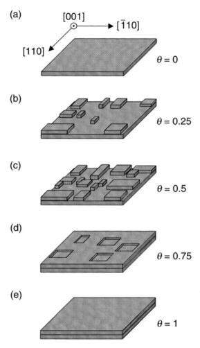
Fig. 3.3. Illustrations of the surface during MBE in 2D-nucleation growth mode.  $\theta$  denotes the surface coverage [8].
