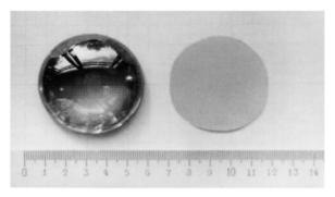
**Fig. 15.9.** ZnSe single crystal grown by a seeded vapor-phase free method in <100> direction and (100) substrate cut from such crystal (from Reference 66)
