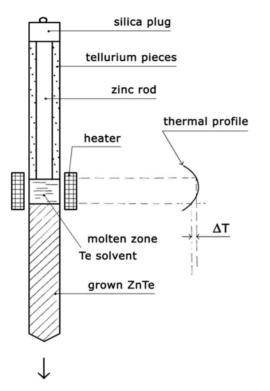
Fig. 15.4. Schematic diagram of "cold THM" principle (from Reference 14)
