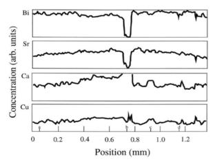
**Fig. 14.38.** Distributions of concentrations of Bi, Sr, Ca, and Cu cations along the line a-d in Fig. 36. EDX was used to obtain this result. A large variation at point b was attributed to the needle crystal of  $(Sr,Ca)CuO_2$ . The high  $T_c$  phase was detected at point c by micro-area X-ray diffractometry. (Reprinted from [34(b)], with permission of Elsevier Science)
