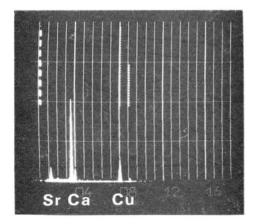
**Fig. 14.5.** X-ray energy dispersive spectrum of the needle crystals in Fig. 14.4(b) (accelerated voltage: 15 kV). (From reference 2 by permission of *Jpn. J. Appl. Phys.*)
