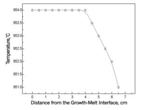
Fig. 12.12. A typical temperature profile of the low thermal gradient furnace
