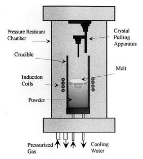
Fig. 15.15. Cermet's melt growth apparatus used for the ZnO growth (from Reference 143)
