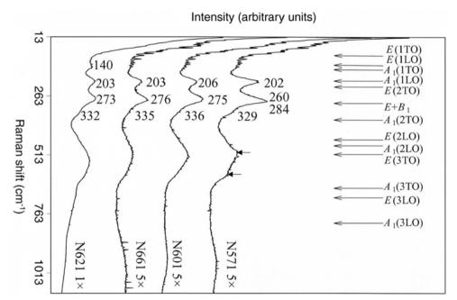
at the top. Fig. 5.7. Raman spectra measured from four PNZT thin films on the MgO substrate. The positions of different Raman peaks at room temperature in  $PbTiO_3$  (Ref. 50) are also shown
