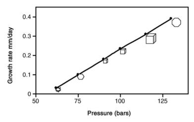
Fig. 10.13. Morphology variation with pressure for Nd:YVO<sub>4</sub> crystals
