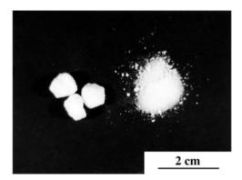
**Fig. 11.2.**  $\alpha$ -cristobalite used as the source material. Right: compacted into lumpus (about 1 cm). Left: compacted into grains (0.5–1.0 mm)
