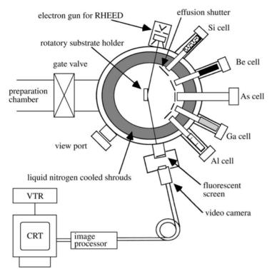
Fig. 3.1. Schematic illustration of the conventional two-chamber MBE
