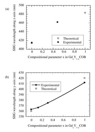
**Fig. 13.15.** Phase-matched wavelength produced by NCPM type-1 SHG along the (a) *z*-axis and (b) *y*-axis of  $Gd_xY_{1-x}Ca_4O(BO_3)_3$  as a function of compositional parameter x
