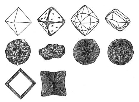
**Fig. 1.4.** Three types of morphologies encountered among natural diamonds. Top four figures show morphologies of single crystalline type, middle four those of polycrystalline type, and the bottom two those of diamond crystals which experienced two different growth parameters
