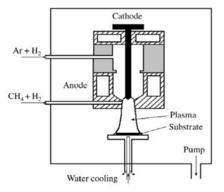
Fig. 4.3. Schematic diagram of the DC arc plasma jet CVD apparatus
