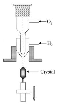
Fig. 17.4. Schematic diagram of Verneuil apparatus
