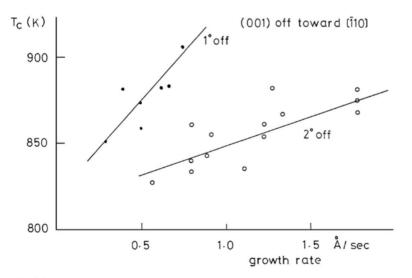
Fig. 3.9. Critical growth temperature for the mode transition vs. growth rate
