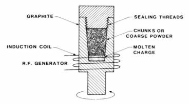
Fig. 15.7. Self-sealing system for the growth of ZnSe crystal (from Reference 48)
