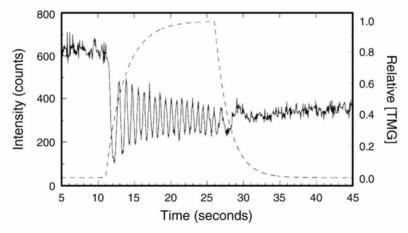
**Fig. 3.19.** CTR intensity during growth. Solid line: intensity of 110 CTR as layer-by-layer growth occurs. Dashed line: Calculated TMG concentration [38]
