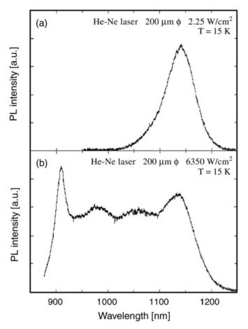
**Fig. 3.26.** PL spectrum from a dot sample that was grown with a deposition time of 3.7 s. The excitation intensities are (a)  $2.25 \text{ W/cm}^2$ , (b)  $6350 \text{ W/cm}^2$  [45]
