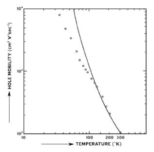
Fig. 15.3. Electron mobility versus temperature for a THM grown ZnTe crystal (from Reference 6)
