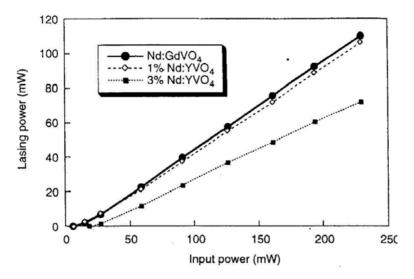
Fig. 10.22. Input-output CW characteristics of Nd:GdVO<sub>4</sub> compared with Nd:YVO<sub>4</sub> [3]
