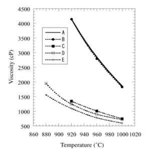
**Fig. 13.20.** Viscosity of solution for KAB crystal growth as a function of temperature for various fluxes. A =  $(K_2CO_3:B_2O_3 = 1:1.8)$ , B =  $(K_2CO_3:B_2O_3:KF = 1:1.8:0.2)$ , C =  $(K_2CO_3:B_2O_3 = 1:1.5)$ , D =  $(K_2CO_3:B_2O_3:LiCl = 1:1.5:0.2)$ , and E =  $(K_2CO_3:B_2O_3:NaF = 1:1.5:0.2)$
