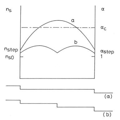
Fig. 3.12. Distribution of the adatom concentration between steps for different step distances
