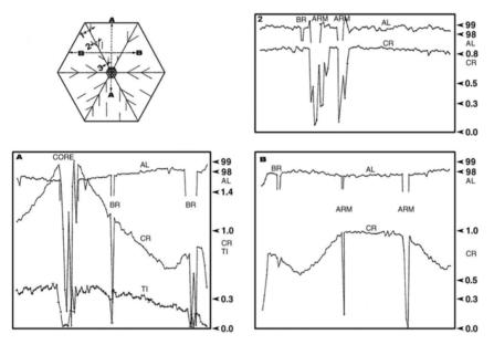
**Fig. 1.13.** Positions of scans A, B, and 1–3 (a), and corresponding plots of microprove analyses of  $Al_2O_3$  (AL),  $Cr_2O_3$  (CR) and  $TiO_2$  (TI). Core indicates opaque core portion, arm and br indicate, respectively, arms and branches [17]
