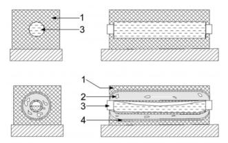
**Fig. 6.2.** Acheson method: (1) unreacted mixture, (2) SiC crystals nucleated in cavities, (3) carbon core with electrodes, and (4) amorphous SiC [25]
