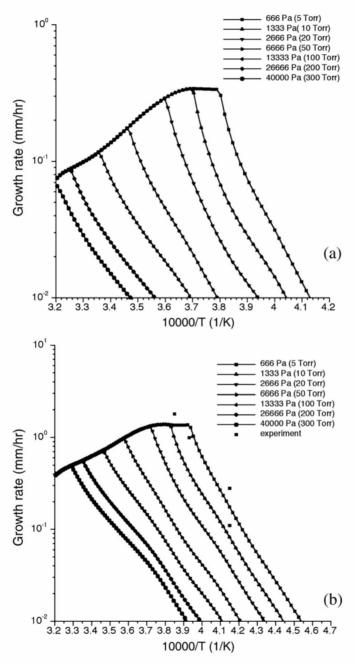
**Fig. 7.12.** Predicted growth rate versus inverse of growth temperature for different gas pressures for axial temperature gradients of (a) 2 K/cm and (b) 20 K/cm [11]. Experimental data for inert gas pressure of 700 Pa in (b) are taken from Nakata et al. [46]
