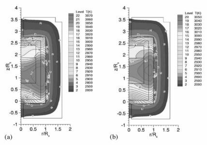
**Fig. 7.10.** Temperature distributions for different coil positions. The coil positions are (a)  $z_{coil} = 0$  and (b) 0.01 m, respectively. The temperature on top of the crucible is kept at 2400 K for all the cases [13].
