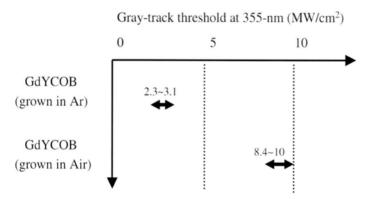
Fig. 13.18. Gray-track threshold of GdYCOB at laser wavelength of 355 nm
