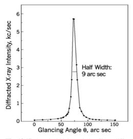
**Fig. 12.17.** A typical high resolution X-ray diffraction curve of a (001) BGO single crystal recorded with (004) planes from the central part of the specimen in symmetrical Bragg geometry
