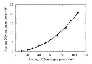
**Fig. 13.10.** Average UV ( $\lambda = 266$  nm) output power as a function of average green input power at 10 kHz. The dotted line is to guide the eyes.
