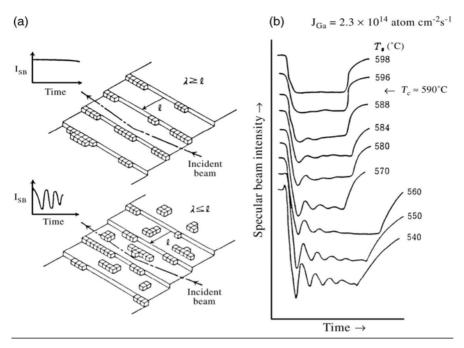
**Fig. 3.7.** Change of growth modes between 2D-nucleation and step flow. (a) Illustrations of the surface for the two modes, (b) RHEED oscillations and growth temperature [10]
