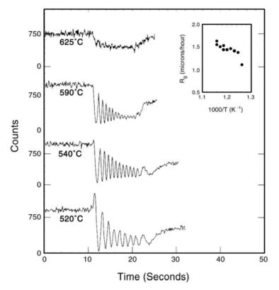
Fig. 3.20. Effect of temperature on layer-by-layer growth. Inset: Arrhenius plot of the temperature-dependent growth rate [38]
