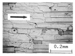
**Fig. 14.21.** PLM photograph (cross-nicols) of a continuous film of the 2212 phase grown on the NdGaO<sub>3</sub> (001) substrate in a period of 10 h. The arrow indicates [100] of NdGaO<sub>3</sub> and [100] of the 2212 phase. (From reference 29 by permission of *J. Crystal Growth*)
