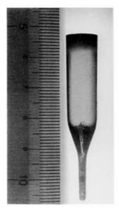
Fig. 15.8. Melt-grown twin-free ZnSe crystal (from Reference 55)
