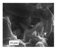
Fig. 11.5. SEM photograph of micro  $\alpha$ -quartz crystals synthesized from sodium formate at a temperature of 300°C
