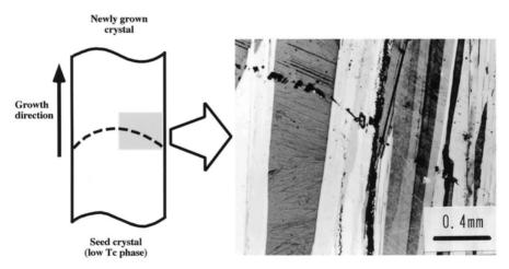
**Fig. 14.40.** Optical micrograph of the section along the growth direction of the rod grown by the TSFZ method with the seed [51]. New crystals continued to grow from the seed crystals.
