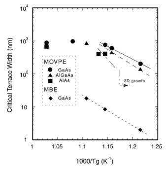
Fig. 3.18. Dependence of the critical terrace width for 2D nuclei generation on the growth temperature [37]
