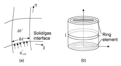
**Fig. 7.3.** (a) Heat flux on the radiation surface and curvilinear grid system, and (b) schematic of ring elements on radiative surfaces. The ring elements coincide with the finite volume grids for conduction calculation [13].
