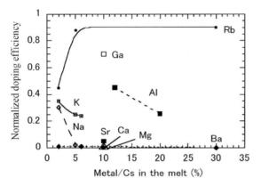
Fig. 13.6. The doping efficiency of various impurities in CLBO crystals as a function of dopant concentration in the melt
