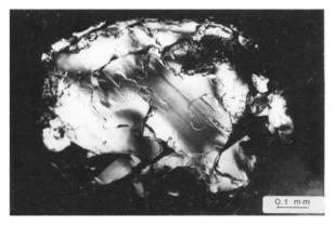
**Fig. 14.11.** Photograph showing the surface microtopograph of the high  $T_c$  single crystal in Fig. 14.9. A differential interference micrograph was used. (From reference 3 by permission of *Jpn. J. Appl. Phys.*)
