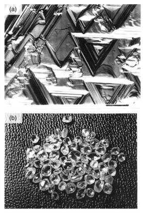
**Fig. 1.7.** DICM photomicrograph of triangular etch pits (trigons) on a (111) face (a). Bar = 0.1 mm. (b) Rounded morphology of natural diamond crystals. Both features are due to dissolution
