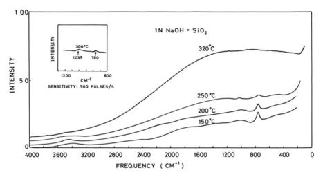
**Fig. 11.12.** Raman spectra of SiO<sub>2</sub>-NaOH-H<sub>2</sub>O system at a series of temperatures. Sensitivity: 1,000 pulses/s
