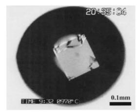
Fig. 14.25. Optical micrograph of the Sm123 crystal coexisting with the liquid in air [37]
