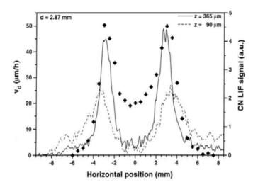
**Fig. 4.14.** Horizontal profiles of the CN LIF signal close to the substrate during diamond growth by an oxyacetylene flame (solid and dashed lines, right-hand ordinate) and the deposition rate  $v_d$  of the corresponding diamond layer along the path of the laser beam (diamonds, left-hand ordinate) [167], *d* is the distance between the flame front and substrate, *z* is the height above the substrate at which the profiles are taken.
