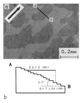
**Fig. 14.18.** (a) Interferogram of the island layers shown in Fig. 14.1a (wavelength: 5470Å). The arrow indicates the direction of either [100] or [010] with respect to the 2212 phase. (b) Sectional view of an island layer on the SrTiO<sub>3</sub> substrate along the line A-B in (a). The dashed line indicates that no information of that part is obtained from the interferogram. (From reference 29 by permission of *J. Crystal Growth*)
