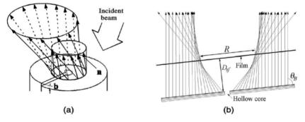
**Fig. 6.10.** The contrast formation mechanism of micropipes on SWBXT back-reflection topographs. (a) Diffraction geometry: *b* is the Burgers vector;  $\vec{n}$  is the position-dependent normal to the (0001) lattice plane; (b) Schematic representation of overlap of the twisted cones in space
