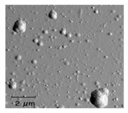
**Fig. 5.2.** AFM micrograph of an amorphous PNZT thin film with thickness of 390 nm after deposition at room temperature. The film was deposited at a laser-beam fluence of 1.0  $J/cm^2$  using 37,500 laser pulses.
