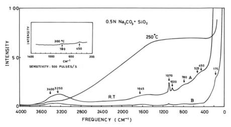
**Fig. 11.13.** Raman spectra of SiO<sub>2</sub>-Na<sub>2</sub>CO<sub>3</sub>-H<sub>2</sub>O system at room temperature and a series of temperatures. Sensitivity: (A) 1,000 pulses/s; (B) 10,000 pulses/s
