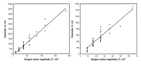
**Fig. 6.7.** Relationship between the magnitudes of screw dislocation Burgers vectors, *b*, and the diameters of the associated hollow cores, *D*. (a) 6H SiC, (b) 4H SiC [79]
