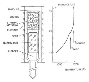
**Fig. 15.10.** Growth ampoule and temperature profile for the growth of ZnSe crystals by a seeded vapor-phase free growth (from Reference 65)
