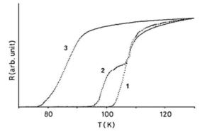
**Fig. 14.3.** Sintering temperature dependence of the *R*-*T* curves for the single high  $T_c$  phase specimen. (1) the original high  $T_c$  phase specimen before heat treatment, (2) 870°C for 1 h, (3) 880°C for 1 h. (From reference 2 by permission of *Jpn. J. Appl. Phys.*)
