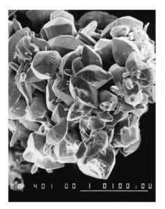
Fig. 11.6. SEM photograph of a crystal group showing Type 1 habit (larger crystals) and Type 2 habit (smaller crystals). 10 wt% NaCl solution, soaked at  $700^{\circ}$ C and quenched at  $650^{\circ}$ C
