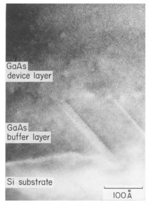
Fig. 3.28. The (011) lattice image of GaAs layer grown on a (001) Si substrate using TCTBL [52]
