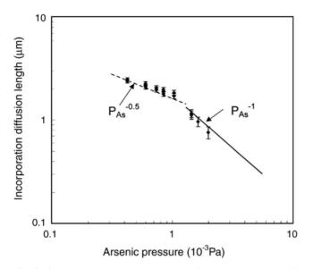
**Fig. 3.13.** Arsenic pressure dependence of the incorporation diffusion length of Ga on the (001) surface. The growth temperature and the side surface were respectively 580°C and (110).
