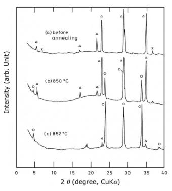
**Fig. 14.14.** X-ray diffraction patterns for the series B single crystals (a) before and (b, c) after annealing in the calcined powder at (b) 850°C and (c) 852°C for 150 h in air. (×) 2201; ( $\Delta$ ) 2212; (Y) 2223. (From reference 4 by permission of *Jpn. J. Appl. Phys.*)
