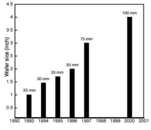
Fig. 6.1. Progress in the increase of diameter of SiC wafers [2]
