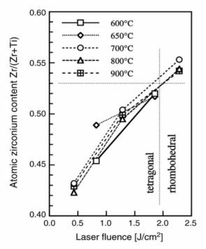
**Fig. 5.4.** Atomic zirconium content, Zr/(Zr+Ti), of PNZT films as a function of laser-beam fluence used at the deposition. The films were post-annealed at various maximum temperatures between 600 and 900°C (reprinted from Ref. 30 with permission from Elsevier Science)
