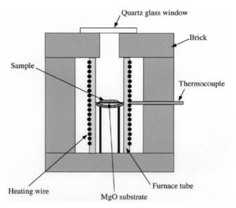
Fig. 14.28. Schematic of the furnace used to scale-up phenomenon under the microscope [37]
