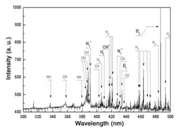
**Fig. 4.17.** Typical optical emission spectroscopy during diamond growth within a  $(N_2 + CH_4 + H_2)$  mixture in the above Hot-Filament Chemical Vapor Deposition diamond apparatus [182]
