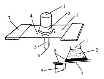
**Fig. 10.4.** Experimental set up for zone melting [17]: (1) polycrystalline feed rod, (2) rod section impregnated by the melt, (3) opening for melt passage, (4) iridium plate, (5) crystal, (6) seed crystal, (7) platinum leads, (8) melt
