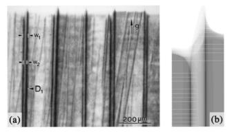
**Fig. 6.16.** Synchrotron transmission topograph showing the double contrast images of micropipes in a longitudinally cut SiC wafer; (b) simulated image of a micropipe in the transmission geometry [99]
