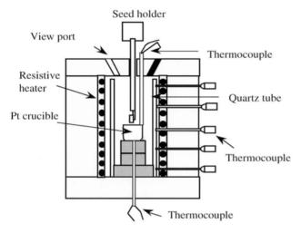
Fig. 13.3. Schematic of a five-zone vertical furnace for top-seeded solution growth of CLBO crystals
