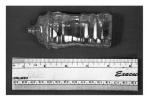
Fig. 12.13. A typical BGO crystal grown by low thermal gradient Czochralski method along the [001] direction
