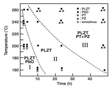
**Fig. 9.4.** TTT (fraction transformation, temperature, time) diagram of  $(Pb,La)(Zr,Ti)O_3$  (PLZT) phase formation under hydrothermal conditions [100]
