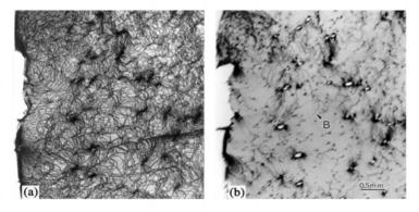
**Fig. 6.23.** (a) Transmission topograph recorded from a basal plane wafer, showing basal plane dislocation loops; (b) the corresponding reflection image, revealing the screw dislocations as well as a few basal plane dislocations [93,122]
