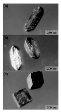
Fig. 10.16(a-c). Characteristic photographs of rare earth vanadate crystals obtained under mild hydrothermal conditions
