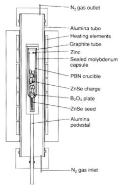
Fig. 15.6. Schematic diagram of the VGF system with the molybdenum Capsule (from Reference 2)  $\,$
