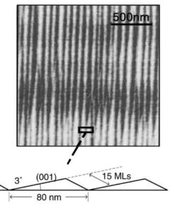
Fig. 3.23. AFM images and cross-section of a thick GaAs buffer layer surface on a vicinal substrate. Observed area is  $1700 \text{ nm} \times 1700 \text{ nm}$  [43]
