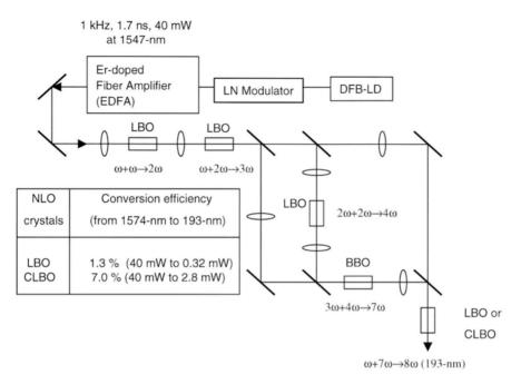
Fig. 13.11. Schematic of experimental set-up for deep-UV light generation at 193 nm
