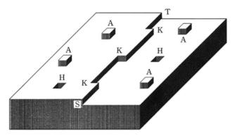
Fig. 2.1. Surface structure of Kossel model
