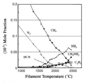
**Fig. 4.11.** Product distribution of major stable gas-phase species as a function of filament temperature measured 4 mm from the filament [150], using 0.5% CH4/0.5% N2 in H2 as the input gas mixture
