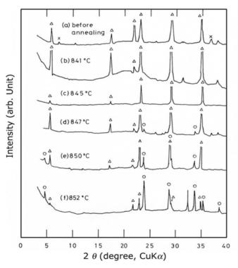
**Fig. 14.13.** X-ray diffraction patterns for the series A single crystals before (a) and after annealing in the calcined  $Bi_2Sr_2Ca_4Cu_6Pb_{0.5}O_y$  powder at (b) 841°C, (c) 845°C, (d) 847°C, (e) 850°C, and (f) 852°C for 150 h in air. (×) 2201; ( $\Delta$ ) 2212; (Y) 2223. (From reference 4 by permission of *Jpn. J. Appl. Phys.*)
