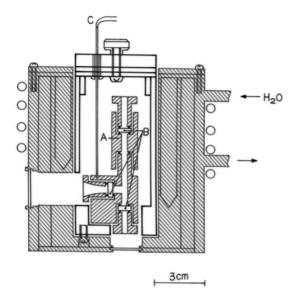
**Fig. 11.10.** Autoclave having optical windows for the measurement of Raman spectra at high temperature and high pressure and electrical furnace. (A) autoclave; (B) sapphire windows; (C) thermocouple
