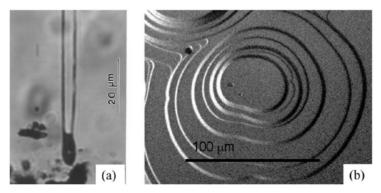
**Fig. 6.20.** (a) Nucleation of a pair of micropipes at an inclusion in 4H-SiC; (b) AFM image showing a typical mesa structure on the growth face of a 4H SiC crystal [112]
