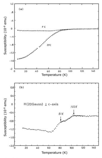
**Fig. 14.10.** Magnetization as a function of temperature for the high  $T_c$  single crystal in Fig. 9. (a) FC: cooling in a field of 20 Gauss, ZFC: cooling in a zero field. (b) This figure shows the same FC data as in (a) except for the units of the vertical axis. The vertical unit is changed from  $10^{-6}$  emu in (a) to  $10^{-7}$  emu in this figure. (From reference 3 by permission of *Jpn. J. Appl. Phys.*)
