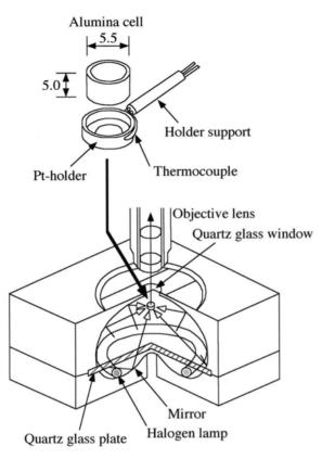
**Fig. 14.24.** Schematic of the infrared heating furnace and the sample cell (Reprinted from [34(c)], with permission of Elsevier Science)
