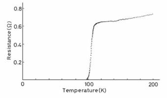
**Fig. 14.9.** Resistivity-temperature curve in the high  $T_c$  single crystal that was found in the bulk sample annealed at 870°C for 100 h in air. (From reference 3 by permission of *Jpn. J. Appl. Phys.*)
