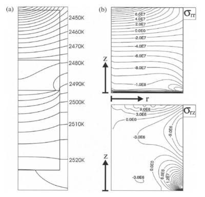
**Fig. 7.19.** (a) Numerical simulation of the axisymmetric temperature distribution inside a growth cell, and (b) resulting thermoelastic stress inside a 6H-SiC crystal: normal stress,  $\sigma_{rr}$ , and shear stress,  $\sigma_{rz}$  (Müller et al. [8])
