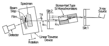
Fig. 12.8. A schematic diagram of the five crystal X-ray diffractometer in the three crystal configuration
