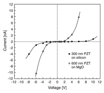
**Fig. 5.10.** Current-voltage characteristics measured at room temperature from a 300 nm thick PNZT film in the Pt/PNZT/Pt structure on the silicon substrate and from a similar structure with a 600 nm thick film on the MgO substrate (reprinted from Ref. 66 with permission from AIP)
