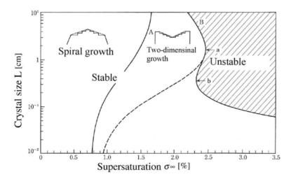
Fig. 2.14. Critical line for stable growth condition
