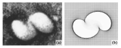
Fig. 6.14. Recorded (a) and simulated (b) images of a micropipe with the same dislocation Burgers vector magnitude and sense [99]
