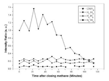
Fig. 4.21. Time evolution of the relative emission intensities after closing methane [182]
