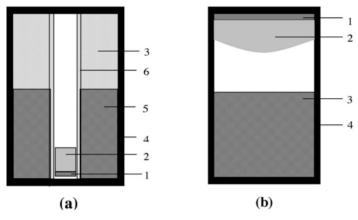
**Fig. 6.4.** Modified Lely method, (a) seed at the bottom, and (b) seed at the top; (1) seed, (2) crystal boule, (3) source material, (4) graphite crucible, (5) graphite powder, (6) porous graphite cylinder
