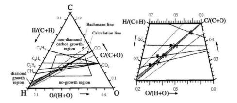
**Fig. 4.8.** Triangular C-H-O diagram for comparison of the diamond domain proposed by Bachmann and the experimental points investigated by Marinelli et al. [132]. The right graph is an enlarged view of the diamond domain region.
