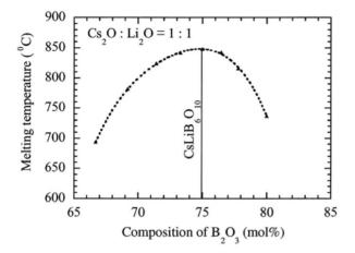
Fig. 13.1. Melting temperatures of the  $(Cs_2O + Li_2O)-(B_2O_3)$  system
