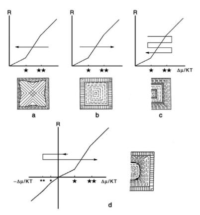
**Fig. 1.2.** Expected internal morphologies in single crystals due to the change of growth parameters during the formation of a single crystal. Arrows in respective R vs.  $\Delta \mu/kT$  diagrams indicate the route of change of driving force conditions during the growth process. Broken lines represent growth banding formed by smooth interface growth, and solid lines dendritic or fibrous textures which appeared by rough interface growth [4]
