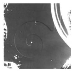
Fig. 6.8. Optical micrograph of a growth spiral on (0001) face of 6H SiC [93]
