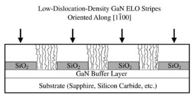
**Fig. 3.30.** Schematic illustration of the MCE process for GaN. The GaN emerging from the window regions has a high density of threading dislocations, whereas the GaN overgrowth on the SiO<sub>2</sub> masks has a drastic reduction in dislocation density [68].
