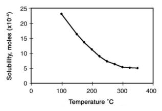
Fig. 10.6. Solubility curve of Nd:RVO<sub>4</sub> in  $1.5 \text{ M HCl} + 3.0 \text{ M HNO}_3$
