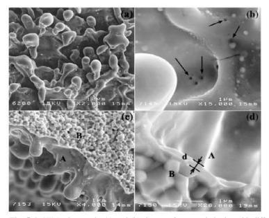
**Fig. 5.6.** SEM micrographs (a) and (b) show surface morphologies with different magnifications and (c) and (d) cross sections of a PNZT target after a scanning laser-ablation process
