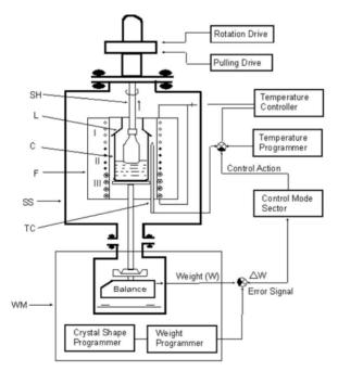
Fig. 12.4. A block diagram of the crystal growth system used for growth of crystals by the low thermal gradient Cz method
