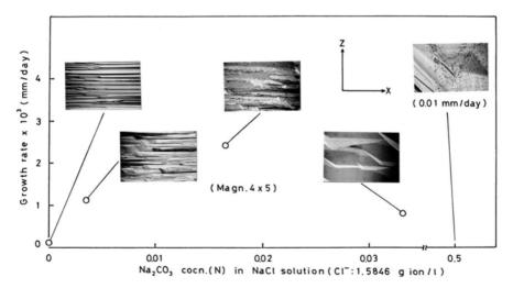
**Fig. 11.1.** Relation between the surface topography on the prism face and  $Na_2CO_3$  conc. (N) in NaCl solution. Growth temp.: 400°C, Dissolving temp.: 425°C, Degree of fill: 70%
