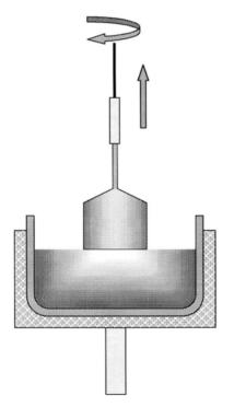
Fig. 17.6. Schematic diagram of Czochralski apparatus
