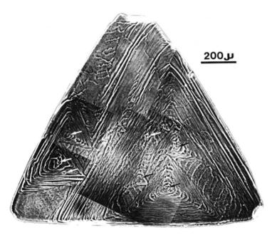
**Fig. 1.6.** Mosaic phase contrast photomicrograph of a (111) face of an octahedral diamond crystal from Siberia, which received only a slight dissolution. Note triangular growth hillocks with the same orientation as the triangle of the (111) face, and a tiny triangular pit (opposite orientation; trigon) at the respective summit of the former growth hillocks. The thinnest growth layers, which consist of growth hillocks, have a step height of less than 0.5 nm. Bar =  $200 \,\mu\text{m}$
