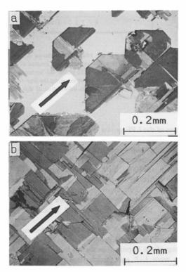
**Fig. 14.17.** PLM photographs (cross-nicols) of the 2212 phase on the SrTiO<sub>3</sub> (100) substrate. (a) Island layers grown in a period of 10 h, and (b) continuous film grown in a period of 22 h. The arrow indicates ( 011) of SrTiO<sub>3</sub> and [100] or [010] of the 2212 phase. (From reference 29 by permission of *J. Crystal Growth*)
