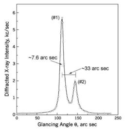
**Fig. 12.21.** A typical high resolution X-ray diffraction curve of a (001) BGO single crystal recorded from the peripheral region of the specimen. (004) diffracting planes were employed
