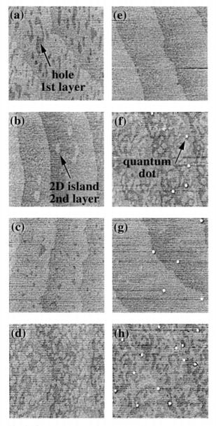
**Fig. 3.25.** AFM images of InGaAs surface grown on GaAs. The deposition times were (a) 0.5 s, (b) 1.0 s, (c) 1.5 s, (d) 2.0 s, (e) 2.5 s, (f) 3.0 s, (g) 3.5 s, and (h) 3.7 s. The scan size of the images was 1  $\mu$ m × 1  $\mu$ m [45].
