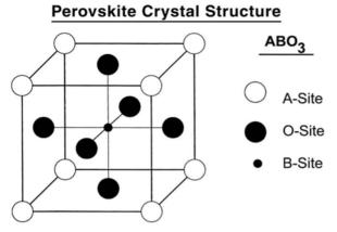
Fig. 9.1. ABO<sub>3</sub> perovskite unit cell [20]
