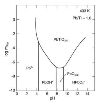
**Fig. 8.1.** Calculated stability diagram for the Pb-Ti system at 433 K.  $PbAc_2$  and  $TiO_2$  are used as starting materials and the ratio of total molalities is equal to 1.0
