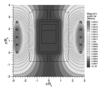
**Fig. 7.6.** magnetic potential contours,  $(A_0)_{real}$ , in a system with a coil of five turns, current of 1200 A and frequency of 10 kHz [13]. Only a portion of the computational domain,  $r \leq 3R_s$  and  $z \leq 4R_s$ , is shown in this figure.
