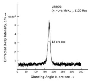
**Fig. 12.14.** A typical high resolution X-ray diffraction curve of a (00.1) LiNbO<sub>3</sub> crystal recorded with (11.0) diffracting planes in symmetrical Laue geometry.  $MoK_{\alpha 1}$  radiation used
