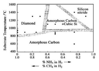
**Fig. 4.15.** Diagram showing the type of films produced on Si substrates after CVD as a function of different substrate temperatures and methane/ammonia ratios. Approximate phase boundaries are included to guide the eye [180]
