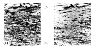
**Fig. 6.17.** Grazing incidence reflection topographs ( $\mathbf{g} = 1126$ ,  $\lambda = 0.70$  Å) recorded from (a) a 6H-SiC substrate before epilayer growth; (b) the same region after growth of a 6  $\mu$ m thick epilayer [109].
