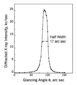
**Fig. 12.18.** A typical high resolution X-ray diffraction curve of a (001) bismuth germanate single crystal recorded with (004) diffracting planes in Bragg geometry when the exploring X-ray beam irradiated the entire specimen along the vertical direction on right hand side of the center.
