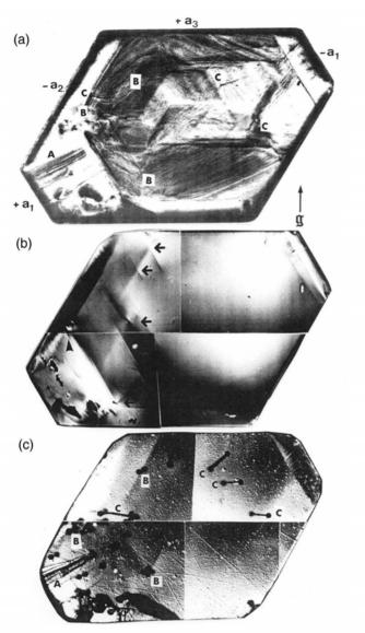
**Fig. 1.9.** X-ray topograph (a) and photomicrographs taken under crossed polarizers before (b) and after (c) etching of a section parallel to the (0001) face of a beryl crystal from Arasuai, Minas Gerais, Brazil. Bar = 1 mm. Arrow with label of g indicates g-vector [12]
