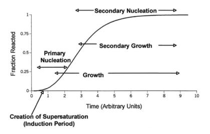
Fig. 9.6. A typical kinetic process for precipitation (fraction reacted vs. time) (After [111])
