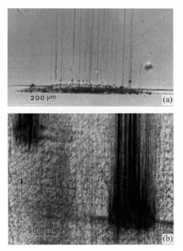
**Fig. 6.19.** (a) Optical micrograph of a part of a (1-100) 4H-SiC wafer showing the nucleation of micropipes at a group of inclusions during growth. (b) SWBXT image recorded in transmission geometry showing the same region as Fig. 6.1(a). (The upper-left region is another group of inclusions at which micropipes nucleate) [112].
