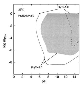
**Fig. 9.2.** Yield diagram for PbTiO<sub>3</sub>. The yield diagram depicts the input concentration of Pb on the *y*-axis and pH on the *x*-axis at the particular temperature of  $25^{\circ}$ C. The shaded region denotes greater than 99% phase-pure PbTiO<sub>3</sub> yield for Pb/Ti molar ratio equal to 2 and Pb/Ti molar ratio equal to 1. The lines represent the beginning of precipitation of PbTiO<sub>3</sub> [20].
