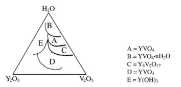
Fig. 10.9. Composition diagram for  $Y_2O_3 - V_2O_5 - H_2O$  system at T = 240°C and 60% fill
