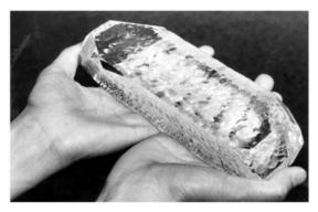
Fig. 17.7. Quartz crystal hydrothermally grown
