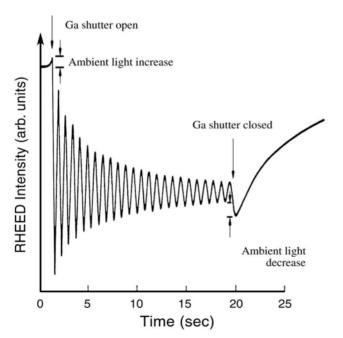
Fig. 3.2. RHEED intensity oscillation observed in MBE of GaAs [8]
