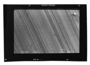
Fig. 15.14. Micro-twins seen on SSR grown ZnS crystals by scanning electron microscopy (from Reference 141)
