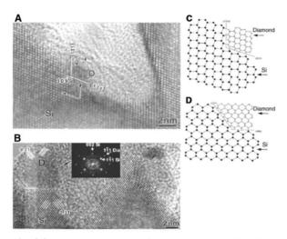
**Fig. 4.4.** (A) HRTEM image of a diamond crystallite (diameter ~2 nm) grown directly on a Si step with an epitaxial alignment. (B) HRTEM image of a diamond crystallite (diameter ~6 nm) grown directly on a Si (001) surface with an epitaxial alignment. (C) and (D) Ball-and-stick diagrams illustrate the interfaces between the diamond crystallites and the Si substrate in (A) and (B) [98].
