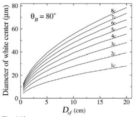
**Fig. 6.12.** Variation of the diameter of the circular micropipe white contrast as a function of the sample-to-film distance  $(D_{sf})$  and the Burgers vector magnitude [99]
