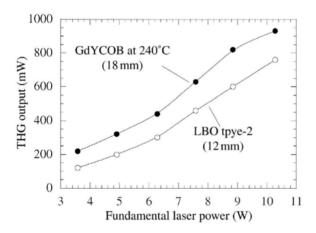
Fig. 13.17. UV output power at 355 nm for two NLO crystals
