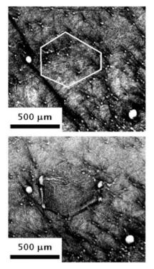
**Fig. 25.** Back-reflection X-ray topographs ( $\mathbf{g} = 00024$ ,  $\lambda = 1.24$  Å) of the area above (a) and below (b) a hexagonal void (a). The projected passage of the void has been traced in white. The screw dislocations visible above the void in (a) are not visible beneath the void in (b) [126]
