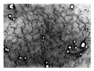
**Fig. 6.9.** SWBXT back-reflection images of close core (smaller white spots) and hollow core (large white spots) screw dislocations in a (0001) 6H SiC wafer. The faint lines connecting these screw dislocation images are basal plane dislocation images [93]
