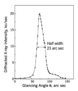
**Fig. 12.19.** A typical high resolution X-ray diffraction curve of a (001) bismuth germanate single crystal recorded with (004) diffracting planes in Bragg geometry from a region on the left hand side of the center.
