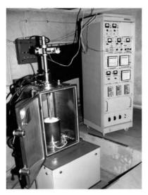
**Fig. 12.3.** A photograph of the crystal growth system employed for growth of crystals by the low thermal gradient Cz method
