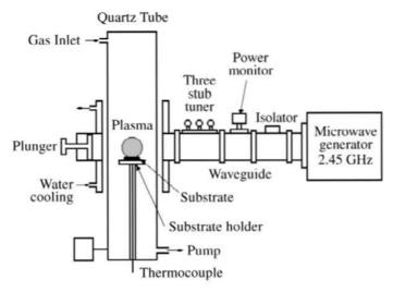
Fig. 4.2. Schematic diagram of the microwave plasma-assisted CVD apparatus
