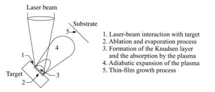
**Fig. 5.1.** Schematic description of different parts of the pulsed-laser-deposition process. In the case of an excimer laser, the pulse duration is around 10 ns and the flight time of the particles from the target to substrate is typically less than 5  $\mu$ s.
