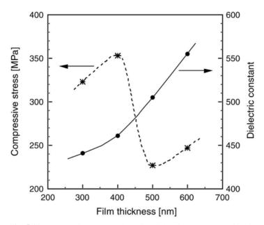
**Fig. 5.11.** Compressive stress and relative dielectric constant as a function of film thickness measured from PNZT films on the MgO substrate (reprinted from Ref. 66 with permission from AIP)
