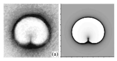
**Fig. 6.21.** (a) SWBXT image recorded in back-reflection geometry from a (0001) Lely platelet showing a pair of opposite-sign screw dislocations; (b) simulation of the image of two opposite-sign screw dislocations ( $b_1 = -b_2 = 12c = 18.2$  nm) with 30 µm spacing. Image dimensions  $200 \times 200$  µm<sup>2</sup> [112]
