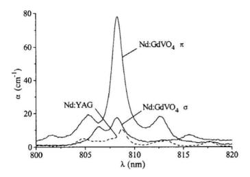
Fig. 10.23. Absorption spectra from the ground state  ${}^{4}I_{3/2}$  into the  ${}^{4}F_{5/2}$  multiplet for Nd:GdVO<sub>4</sub> in  $\pi$ - and  $\sigma$ -polarization [23]
