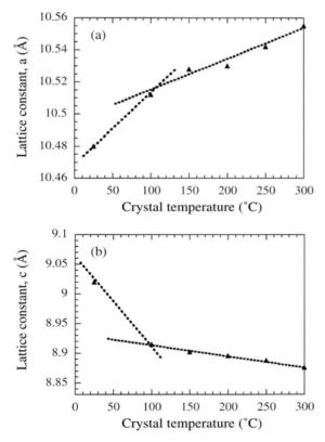
**Fig. 13.8.** (a) Elongation of CLBO lattice constant along the *a*-axis and (b) contraction of CLBO lattice constant along the *c*-axis
