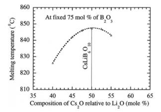
Fig. 13.2. Melting temperatures of the (Cs<sub>2</sub>O)-(Li<sub>2</sub>O) system at 75 mole % of B<sub>2</sub>O<sub>3</sub>
