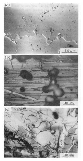
**Fig. 14.16.** Photographs showing the surface microtopographs of the series B crystals (a) before and (b, c) after annealing at (b) 850°C and (c) 852°C. (From reference 4 by permission of *Jpn. J. Appl. Phys.*)
