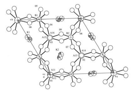
Fig. 13.19. Projection of the KAB crystal along the (a) *a*-axis and (b) *c*-axis
