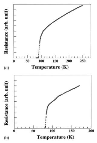
**Fig. 14.32.** Temperature dependence of the resistance of the sample grown from a high-temperature solution. a) As-grown sample. (b) The sample annealed at  $800^{\circ}$ C in oxygen atmosphere for one day. (Reprinted from [34(a)], with permission of Elsevier Science)
