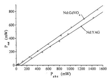
Fig. 10.20. Diode-laser pumped lasing of  $Nd:GdVO_4$  and Nd:YAG at 1.06  $\mu$ m under identical conditions [23]
