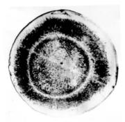
**Fig. 12.15.** A typical high resolution X-ray diffraction traverse topograph of an unpoled (00.1) LiNbO<sub>3</sub> crystal recorded in symmetrical Laue geometry with (11.0) diffracting planes and MoK<sub> $\alpha$ 1</sub> radiation
