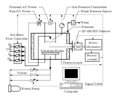
Fig. 4.16. Schematic diagram of experimental apparatus useful for spatially resolved optical emission spectroscopy [181]
