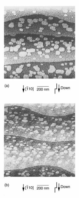
**Fig. 3.17.** STM images showing the denuded zones near steps and the 2D nuclei of (a) GaAs and (b) AlAs. About a 1/6 ML of GaAs or AlAs was deposited on a very flat (001) GaAs surface at  $630^{\circ}$ C [36].
