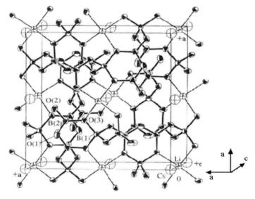
Fig. 13.5. Molecular packing of CLBO in a three-dimensional framework
