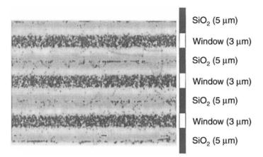
Fig. 3.31. CL image of a GaN MCE layer for which coalescence at the centers of the  $SiO_2$  masks is completed [68]
