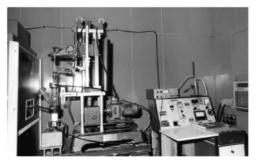
Fig. 12.1. A photograph of a crystal growth system designed and developed at NPL (National Physical Laboratory, New Delhi, India)
