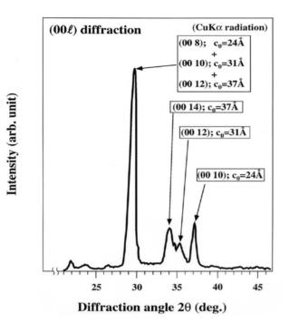
**Fig. 14.37.** X-ray profile at the point c in Fig. 14.36 obtained by micro-area X-ray diffractometry. The size of the incident beam was 50  $\mu$ m in diameter. (Reprinted from [34(b)], with permission of Elsevier Science)
