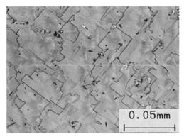
**Fig. 14.20.** Continuous film of the 2201 phase grown on the (100) face of the LaA1O<sub>3</sub> substrate (DIM micrograph). The film thickness was about 1  $\mu$ m. (From reference 29 by permission of *J. Crystal Growth*)
