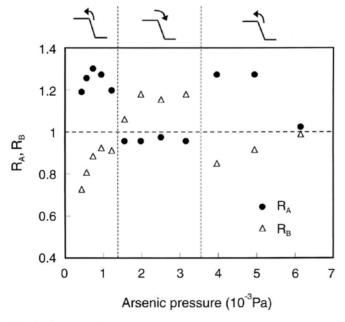
**Fig. 3.15.** Normalized growth rate on (001) near the boundary and that on (111)B vs. arsenic pressure.  $R_A = R_{comer}^{(001)} / R_{comer}^{(001)}$  and  $R_B = R_{comer}^{(111)B} / R_{planar}^{(111)B}$
