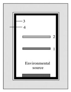
**Fig. 6.5.** Sublimation sandwich method: (1) source wafer, (2) substrate, (3) graphite container, and (4) insulation material
