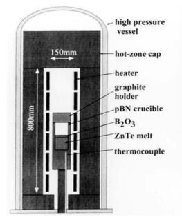
Fig. 15.2. High pressure VGF furnace (from Reference 9)
