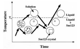
Fig. 14.26. Diagram of the self-seeding technique and determination of the liquidus temperature [37]
