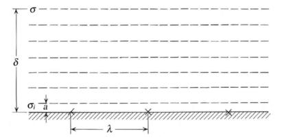
Fig. 2.9. Distribution of supersaturation for the surface diffusion model by Bennema. There are steps at the cross point.
