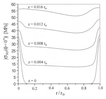
**Fig. 7.20.** Radial dependence of the resolved shear stress in the < 1120 > direction at different distances from the growth interface (z = 0) (Müller et al. [8])
