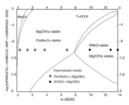
Fig. 8.6. Stability of various solid phases in the Pb-Mg-Nb-K-H<sub>2</sub>O system at 473 K
