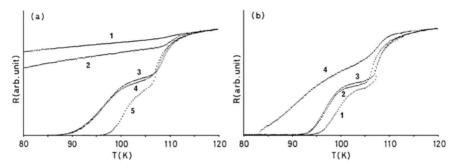
**Fig. 14.1.** Sintering temperature dependence of the *R*-*T* curves for specimens that were sintered at various temperatures for 30 h in a stream of  $\text{Ar-O}_2$  gas of about 1 atm with an oxygen partial pressure of 1/13 atm: (a) (1) 790°C, (2) 800°C, (3) 810°C, (4) 820°C, (5) 830°C; (b) (1) 840°C, (2) 855°C, (3) 860°C, (4) 870°C. (From reference 2 by permission of *Jpn. J. Appl. Phys.*)
