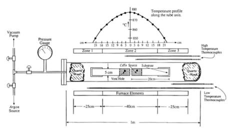
Fig. 15.11. SPVT system used by Eagle Picher for the growth of CdTe and ZnSe (from Reference 83)
