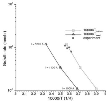
**Fig. 7.13.** Dependence of the growth rate on the seed temperature,  $T_{seed}$ , and the temperature on the bottom of the crucible,  $T_{bottom}$  in a 75 mm system [15]. The symbols from top to bottom correspond to currents of 1200 A, 1100 A, and 1000 A, respectively. Experimental data are taken from Balkas et al. [42]
