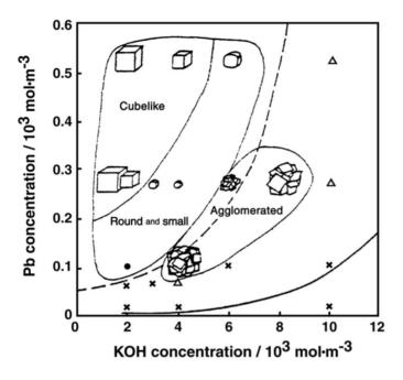
**Fig. 9.9.** Schematic representation of the morphology of Pb(Zr,Ti)O<sub>3</sub> powders synthesized at 150°C for 4 hours. Solid line and dashed line are for the Pb concentration saturated with PbO and Pb(Zr,Ti)O<sub>3</sub> powder, respectively. Phases of Pb(Zr,Ti)O<sub>3</sub> ( $\lambda$ ), and Pb(Zr,Ti)O<sub>3</sub> with other crystalline solids (triangles), and amorphous (**x**) [99]
