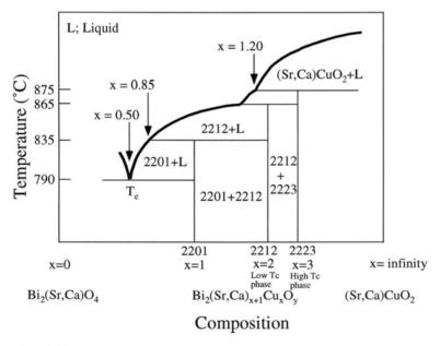
**Fig. 14.34.** The pseudo-binary phase diagram of  $Bi_2(Sr,Ca)_{x+1}Cu_xO_y$  proposed after *in situ* observation.  $Bi_2(Sr,Ca)O_4$  at x = 0 and  $(Sr,Ca)CuO_2$  at x = infinity (Reprinted from [34(a)], with permission of Elsevier Science)
