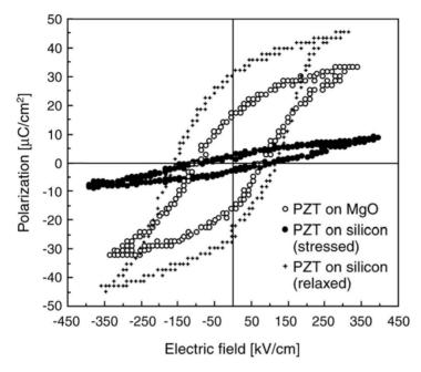
**Fig. 5.9.** Polarization vs. electric field hysteresis loops of the Pt/PNZT/Pt capacitor structures on MgO and silicon substrates. In the case of the silicon substrate, hysteresis loops measured from both stressed and relaxed PNZT films are shown (reprinted from Ref. 66 with permission from AIP)
