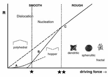
Fig. 1.1. Morphologies of single crystals (polyhedral, hopper, dendritic) and polycrystalline aggregates (spherulitic and fractal) in relation to growth rate R, driving force, interface roughness (smooth and rough) and growth mechanisms. Curve *a* represents the spiral growth, curve *b* the two-dimensional nucleation growth, and curve *c* adhesive-type growth mechanisms. The critical points \* and \*\* are the points where the predominant growth mechanism changes [4]
