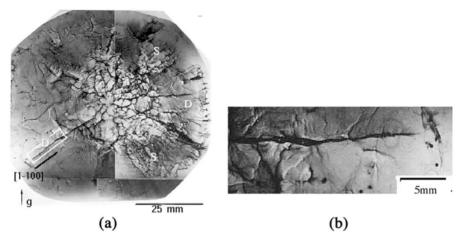
**Fig. 6.24.** (a) Back-reflection topograph of experimental 3-inch 4H-SiC wafer [(00016),  $\lambda = 1.26$  Å] showing several small angle boundaries; (b) enlargement from framed section on Fig. 6.17(a), clearly showing the orientation contrast (image overlap) from one of the boundaries [122]
