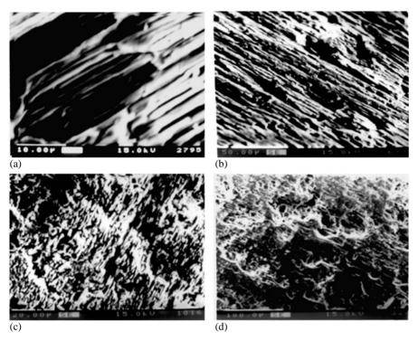
Fig. 10.18(a-d). Surface dissolution features in rare earth orthovanadate crystals
