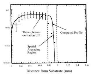
**Fig. 4.13.** Atomic hydrogen atom concentration profile measured using three-photonexcitation LIF in stagnation-flow diamond-forming flame apparatus [163]
