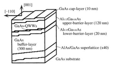
Fig. 3.22. Schematic illustration of a QWW structure on a GaAs vicinal substrate [43]
