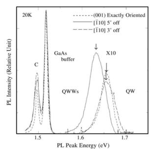
Fig. 3.24. Photoluminescence spectra of QWW structures [43]
