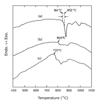
**Fig. 14.12.** DTA heating curves for (a) the calcined powder of  $Bi_2Sr_2Ca_4Cu_6Pb_{0.5}O_{y}$ , (b) the series A crystals, and (c) the series B crystals before annealing experiments (heating rate; 10°C/min). Arrows indicate the range of annealing temperatures used in this study (841~852°C). (From reference 4 by permission of *Jpn. J. Appl. Phys.*)
