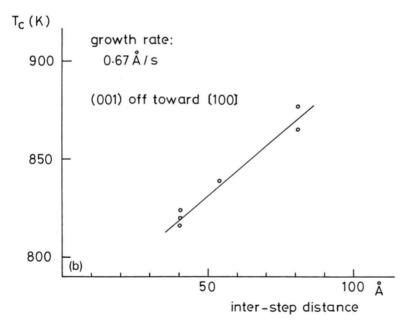
Fig. 3.11. Critical growth temperatures for the mode transition vs. step distance
