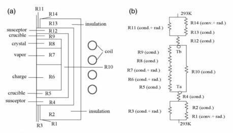
**Fig. 7.2.** (a) Schematic and (b) thermal network of a SiC growth system (cond. — conduction, conv. — convection, rad. — radiation) [10]
