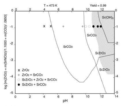
**Fig. 8.10.** Calculated phase stability and yield diagram at 473 K for Sr/Zr = 1.1 using  $Sr(NO_3)_2$  as a source of strontium when the amount of  $CO_2$  in the starting materials is equal to 0.085 times the amount of  $ZrO_2$ . The symbols denote experimental conditions for which the following products were obtained: (x)  $ZrO_2$ , (+)  $SrCO_3 + ZrO_2$ , ( $\Upsilon$ )  $SrZrO_3 + ZrO_2 + SrCO_3$ , ( $\bullet$ )  $SrZrO_3 + SrCO_3$
