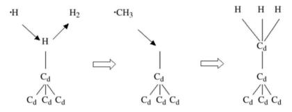
Fig. 4.5. A possible reaction schemes for the growth of CVD diamond film
