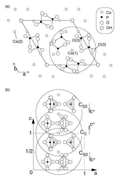
**Fig. 16.1.**  $Ca_9(PO_4)_6$  cluster unit,  $C_0$  and  $C_{50}$ , projected on the *ab* plane (a) and *ac* plane (b) of the hydroxyapatite. Because both cluster units have only  $C_3$  symmetry (noncentrosymmetric) and are related by mirror planes at z = 1/4 and 3/4, they are chiral. (Reprinted with permission from Onuma, K., Ito, A. *Chemistry of Materials*, 10:3346–3351 (1998). Copyright 1998 American Chemical Society.)
