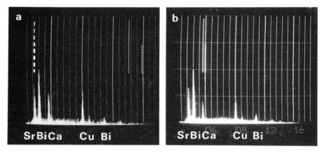
**Fig. 14.6.** Comparison of the composition of high  $T_c$  crystals with that of low  $T_c$  crystals using X-ray energy dispersive spectra. The X-ray system used 15 kV. a) High  $T_c$  (A in Fig. 14.4a); b) Low  $T_c$  (C in Fig. 14.4b). (From reference 2 by permission of *Jpn. J. Appl. Phys.*)
