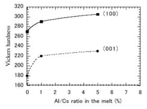
Fig. 13.7. Vickers hardness of Al-doped CLBO (100) and (001) surfaces as a function of Al/Cs ratio in the growth melt
