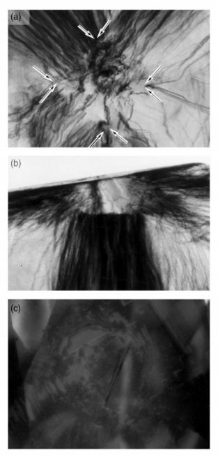
**Fig. 1.5.** X-ray topographs (a and b) and cathodoluminescence tomograph (c) of core portion of a round (a) and pear-shaped (b and c) brilliant cut diamonds. (a) and (b) are plan and profile views, respectively, (c) is a plan view. White arrows in (a) indicate the boundary of the core portion [10]
