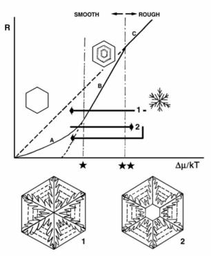
**Fig. 1.14.** Schematic diagram showing two routes 1 and 2 for trapiche ruby without (route 1) and with clear ruby core (route 2), superimposed on Fig. 1.1 [17]
