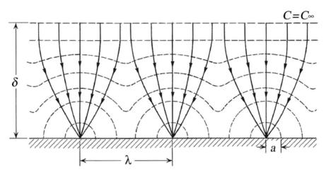
Fig. 2.8. Distribution of concentration for the volume diffusion model. The dotted line is the isosbestic line.
