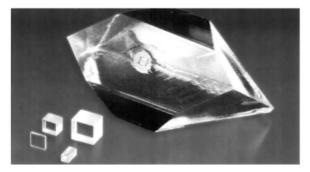
Fig. 13.4. Photograph of a large CLBO crystal with dimensions of  $14 \times 11 \times 11$  cm<sup>3</sup>
