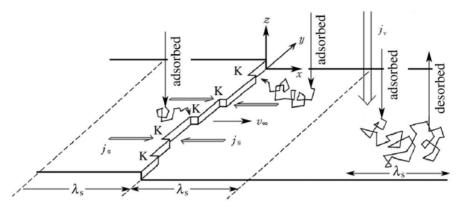
Fig. 2.3. Motion of a step and adatoms
