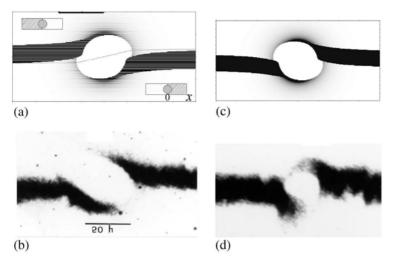
**Fig. 6.13.** Section topographs showing the senses of screw dislocations associated to micropipes. (a) and (b) are the simulated and recorded images of a right-handed screw dislocation, respectively; (c) and (d) are the simulated and recorded images of a left-handed screw dislocation [98]
