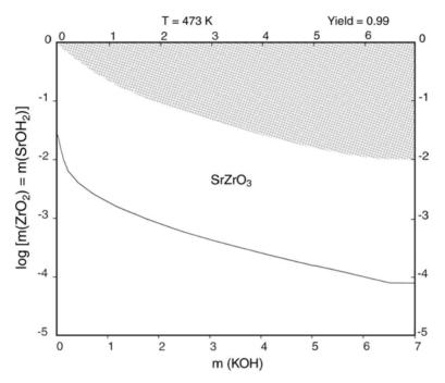
**Fig. 8.5.** Calculated phase stability and yield diagram as a function of the input amount of KOH at 473 K for Sr/Zr = 1 using  $Sr(OH)_2$  as a source of strontium
