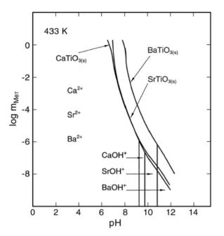
**Fig. 8.2.** Comparison of calculated phase stability diagrams for the hydrothermal systems Ca-Ti, Sr-Ti, and Ba-Ti at 433 K for the stoichiometric molar ratios of precursors
