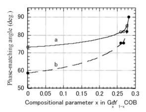
**Fig. 13.14.** Changes of phase-matching angles for THG as a function of the compositional parameter x
