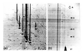
**Fig. 1.11.** (a) Photomicrograph of tube-like two-phase inclusions formed behind solid inclusions indicated by arrows. (b) Strain field (arrow A) around a dislocation generated from a misfit in the incorporation of the inclusion and negative growth banding (arrows X). LI is a two-phase inclusion [12]
