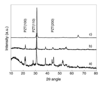
**Fig. 5.3.** XRD patterns from PNZT films deposited on the sapphire substrate at laser-beam fluences of (a) 0.4 (annealed at 850°C), (b) 1.3 (annealed at 850°C) and (c) 2.4 J/cm<sup>2</sup> (annealed at 800°C). The intensity values of the curve (c) were divided by a factor of 10 as compared with the intensity values of other curves (Reprinted from Ref. 30 with permission from Elsevier Science)
