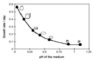
Fig. 10.15. Morphology variation with pH for Nd:  $YVO_4$  crystals obtained from sintered nutrient
