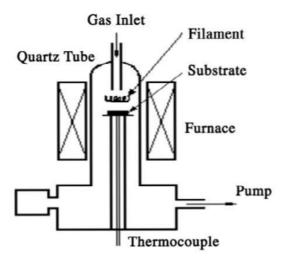
Fig. 4.1. Schematic diagram of the hot-filament CVD apparatus
