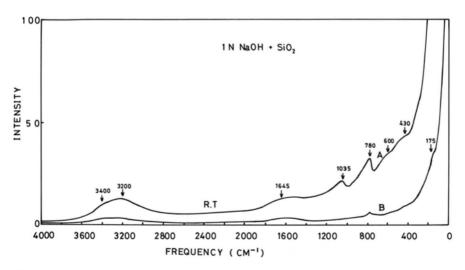
**Fig. 11.11.** Raman spectra of SiO<sub>2</sub>-NaOH-H<sub>2</sub>O system at room temperature. Sensitivity: (A) 1,000 pulses/s; (B) 10,000 pulses/s
