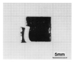
Fig. 14.29. Photograph of the Sm123 crystal grown by the self-seeding technique under the large furnace [37]
