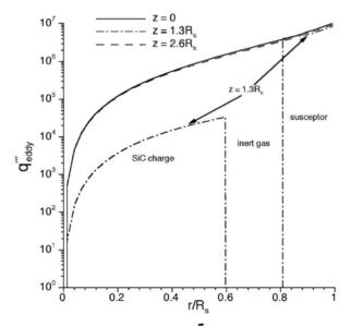
**Fig. 7.7.** Generated heat power,  $q_{eddy}^{"}$ , along the radial direction at different heights z = 0,  $1.3R_s$ , and  $2.6R_s$ . The profile at  $z = 1.3R_s$  has an inert gas gap between the powder charge and the susceptor [13].
