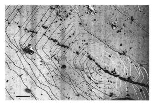
**Fig. 1.8.** DICM photomicrograph of elemental growth spirals on (0001) face of a beryl crystal from Minas Gerais, Brazil. Bar = 500  $\mu$ m. Small dots are etch pits selectively formed at dislocation outcrops [12]
