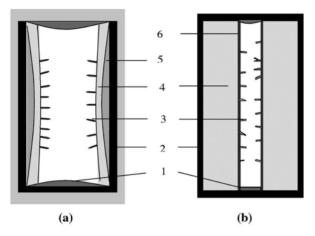
**Fig. 6.3.** (a) Original Lely method, (b) Improved Lely method; (1) SiC deposit, (2) graphite crucible, (3) SiC platelets, (4) SiC lump, (5) carbon from decomposed SiC, (6) graphite porous cylinder
