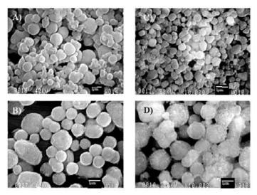
**Fig. 9.8.** SEM micrographs of precursors of spherical titania with particle size of (a) 1  $\mu$ m, (b) 1.5  $\mu$ m, and respective product of (Ba,Sr)TiO<sub>3</sub> with corresponding particle sizes (c) 1  $\mu$ m, (d) 1.5  $\mu$ m
