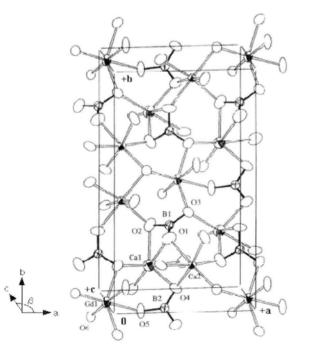
Fig. 13.12. Molecular packing of GdCOB in a three-dimensional framework
