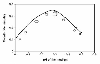
Fig. 10.12. Dependence of growth rate and pH of the growth media for  $Nd:GdVO_4~1.0~M$   $HCl+1.0~M~HNO_3$
