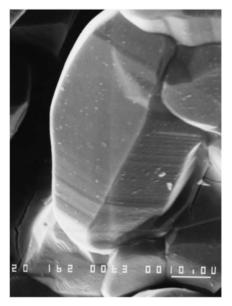
Fig. 11.8. SEM photograph of  $\beta$ -quartz crystal (Type 2F). 1 N NaOH solution, soaked at 750°C, and quenched at 700°C
