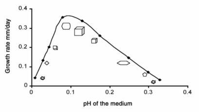
Fig. 10.11. Dependence of growth rate and pH of the media for Nd:YVO<sub>4</sub> 1.5 M HCl + 3.0 M HNO<sub>3</sub>
