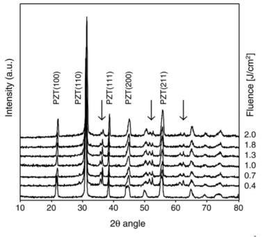
**Fig. 5.5.** X-ray diffraction patterns measured with  $\text{CuK}\alpha$  radiation (1.54 Å) from a PNZTtarget surface before and after scanning laser ablation with various laser-beam fluences between 0.4 and 2.0 J/cm<sup>2</sup>. The arrows indicate three twin peaks from a new phase (tetragonal ZrO<sub>2</sub>) formed in the laser-ablation process.
