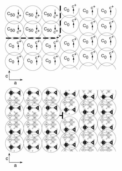
**Fig. 16.2.** A edge dislocation with Burgers vector of C/2 formed by stacking fault of  $C_0$  and  $C_{50}$  clusters. The interface between  $C_0$  domain and  $C_{50}$  domain is perpendicular to the *c*-axis, and the C<sup>+</sup> direction of each domain is anti-parallel.
