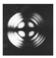
**Fig. 12.11.** A conoscopic interferrogram for white light of LiNbO<sub>3</sub> sample cut perpendicular to the growth axis
