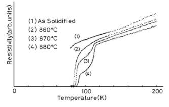
**Fig. 14.7.** Annealing temperature dependence of the *R*-*T* curves for the bulk samples that were prepared by slowly cooling the melt of Bi:Sr:Ca:Cu = 4:3:3:4. The samples were annealed at 860–870°C in air for 50 h. (From reference 3 by permission of *Jpn. J. Appl. Phys.*)
