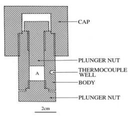
Fig. 11.4. Schematic diagram of hydrothermal hot-press
