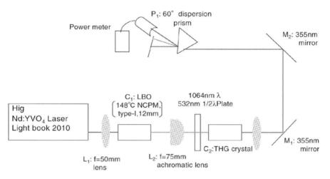
Fig. 13.16. Experimental set-up for high-repetition rate THG measurement
