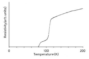
**Fig. 14.8.** Resistivity-temperature curve in the bulk sample that was annealed at 870°C for 100 h in air. (From reference 3 by permission of *Jpn. J. Appl. Phys.*)
