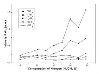
Fig. 4.19. Effect of nitrogen concentration on the relative emission intensities [182]
