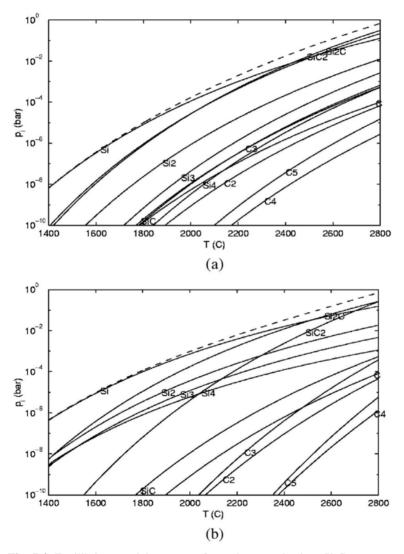
**Fig. 7.4.** Equilibrium partial pressures for various species in a Si-C system assuming (a) condensed SiC and carbon, (b) condensed SiC and silicon. The dashed line is the total pressure [19].
