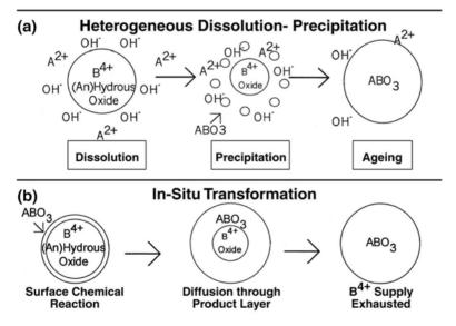
Fig. 9.5. Two mechanisms: (a) dissolution-precipitation and (b) *in situ* transformation (After [2])
