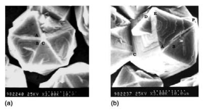
**Fig. 4.6.** Scanning electron micrographs of diamond film. (a) A five-fold twin partical. Facets B and C show right- and left-handed spirals, respectively. (b) A multiply twinned particle. Facet A shows some terraces by step flow growth mode; facet B shows a spiral growth [107].
