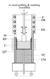
Fig. 12.2. A schematic line diagram of the crucible set-up of the crystal growth system developed at NPL
