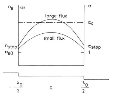
Fig. 3.10. Distribution of the adatom concentration between steps for different Ga fluxes
