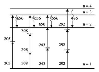
Fig. 4.12. Energy level schematic for various multiphoton-excitation LIF techniques for the measurement of atomic hydrogen concentration [163]
