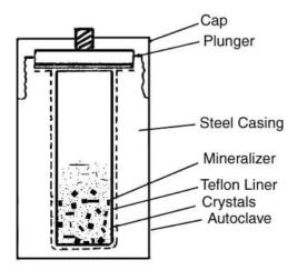
Fig. 10.10. Schematic diagram of the hydrothermal autoclave
