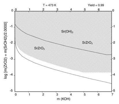
**Fig. 8.8.** Calculated phase stability and yield diagram as a function of the input amount of KOH at 473 K for Sr/Zr = 2.0 using  $Sr(OH)_2$  as a source of strontium. The solid circle denotes experimental conditions for which phase-pure  $SrZrO_3$  was obtained.
