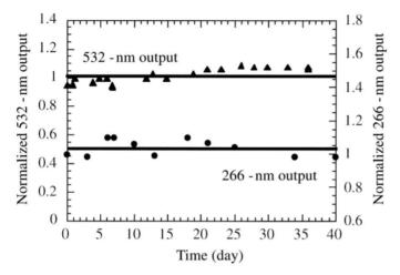
**Fig. 13.9.** Normalized output energy at 532 and 266 nm from CLBO crystals at 160°C. Stable performance was obtained for more than one month with continuous exposure to ordinary room humidity.
