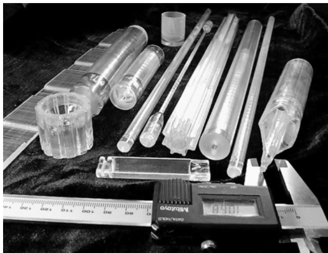
Figure 5.13 Sapphire shaped crystals grown by the VST.
