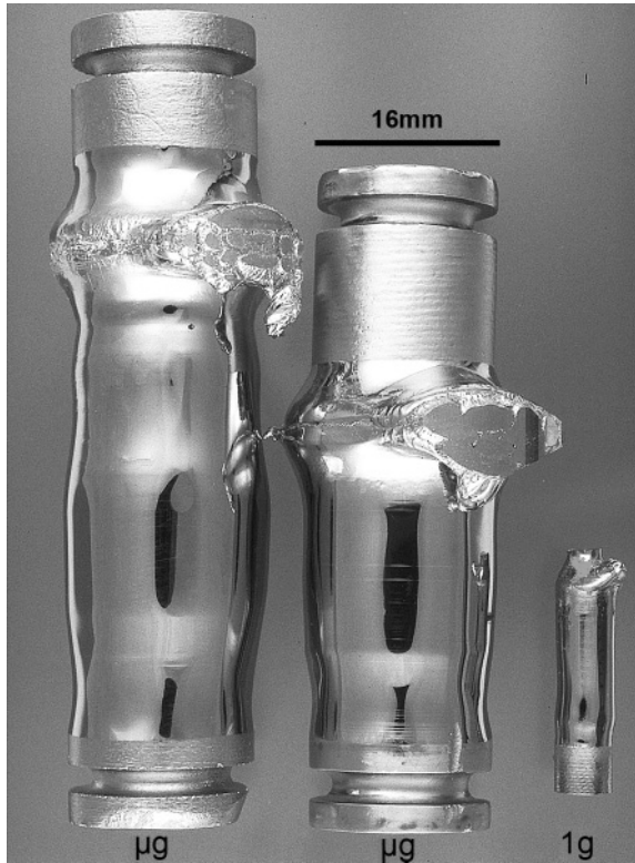
Figure 4.28 Two GaSb crystals of 16 mm diameter grown under microgravity (left and centre) during the Spacehab-4 mission [Tegetmeier 1996], and one 5-mm diameter GaSb crystal grown under gravity (right) (copyright A. Cröll and R. Geray; reproduced with permission).
