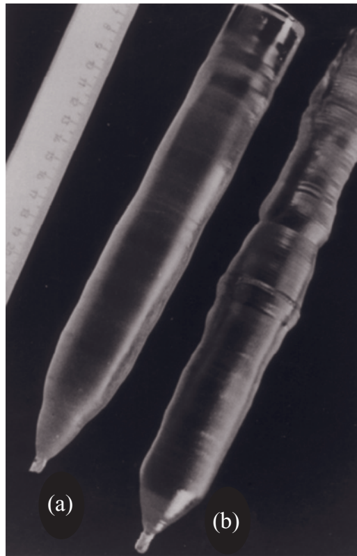
Figure 2.14 Corundum crystals grown by the Verneuil technique with automatic regulation under stable (a) and unstable (b) laws of powder charge control.
