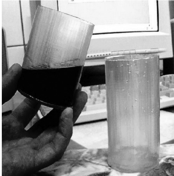
Figure 5.22 Sapphire crucibles of 65 mm in diameter grown by the NCS technique.
