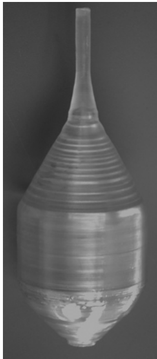
Figure 5.28 Sapphire hollow crystal grown by the GES technique.
