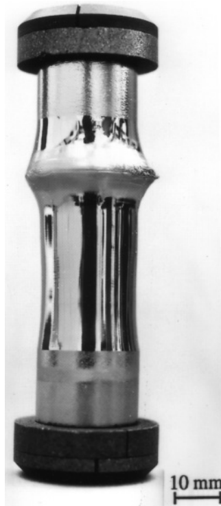
Figure 4.29 20-mm diameter GaAs FZ crystal grown under microgravity during the German Spacehab mission D-2 in 1993 (Reprinted with permission from [Herrmann 1995], copyright (1995) Elsevier Ltd).
