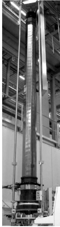
Figure 5.3 EFG growth furnace at RWE SCHOTT Solar with growing thin-walled octagonal Si tube (Reprinted with permission from [Behnken 2005], copyright (2005) Elsevier Ltd).
