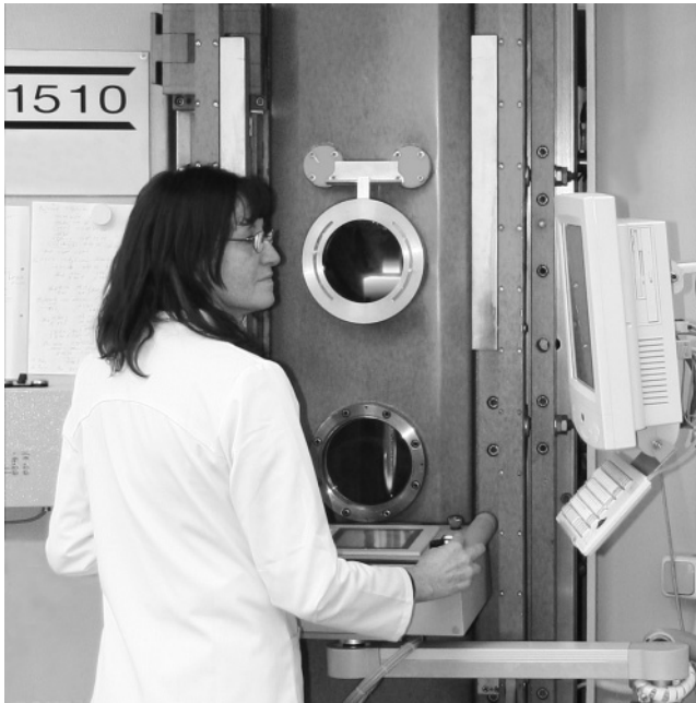
Figure 4.12 FZ machine in operation (pedestal experiment); large windows for process observation are available at the front and on both sides.
