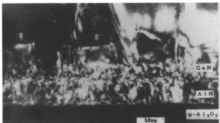
Figure 6. Bright field image with a low magnification to observe a wide region of a GaN epitaxial layer with an AlN buffer layer.
