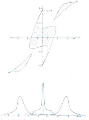
FIG. 2. (Upper) phase space of light transmitted by the polarizing system, determined along the line X-X in Fig. 1. The calculated phase space is outlined, the observed phase space is hatched, and the two polarizations are oppositely hatched.  $\theta$  is the angle between a light ray and the axis of the instrumert. (Lower) plot of the intensity of light of the two polarizations along the line X-X in Fig. 1.
