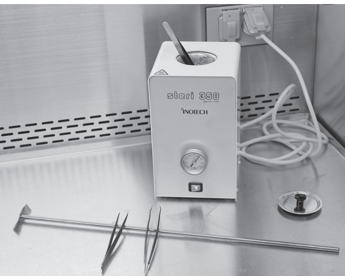
Figure 4-10. A glass bead sterilizer.
