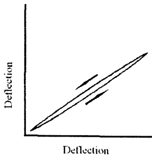
Figure 2.18. Hysteresis in the response of a piezoelectric tube scanner between forward and reverse directions.
