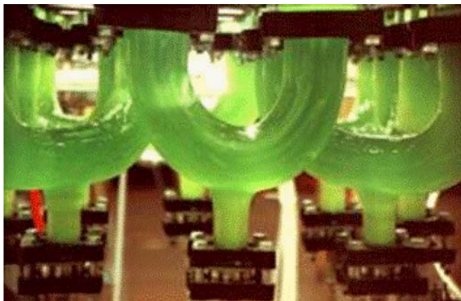
Fig. 1 Loops of a 100 l “Medusa”-photobioreactor under operation conditions, working via recirculation of synthetic sea water via continuous aeration of one tube of the loops. (Pictures kindly provided by Christian Walter, see [85])
